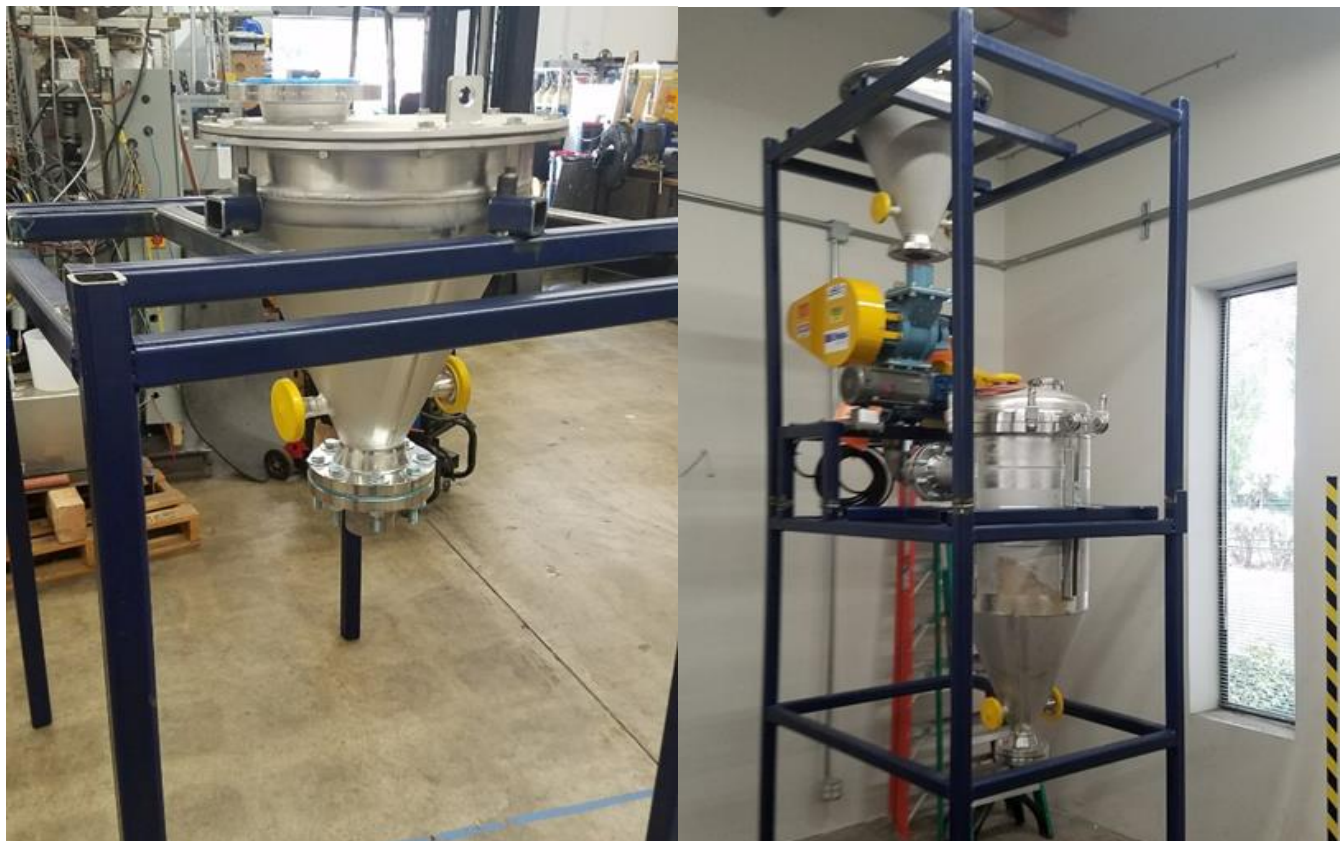
Figure 33: Installed Upper Hopper (Left) and Completed Feed System (Right)
