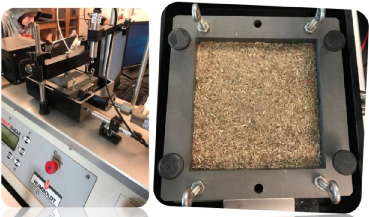
Figure 16: Direct Shear Test Unit for Measuring Shear Stress
