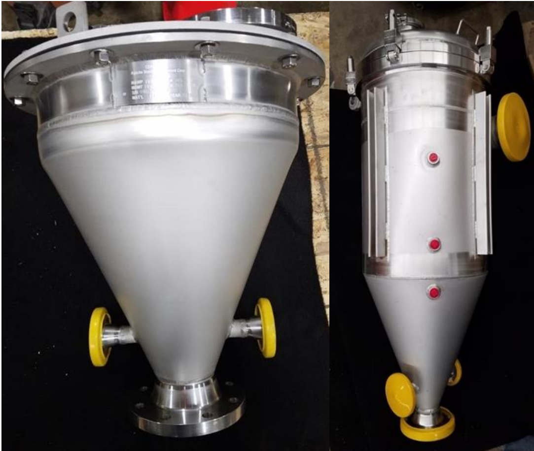
Figure 28: Upper (Left) and Lower (Right) Hoppers
