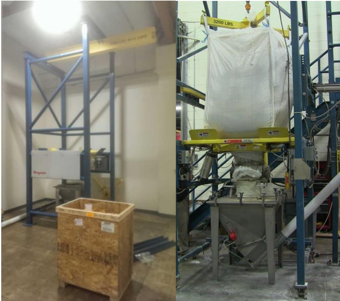
Figure 27: Photograph of the Bulk-Bag Unloader During Assembly at Altex (Left) and During Testing at Supplier's Facility (Right)
