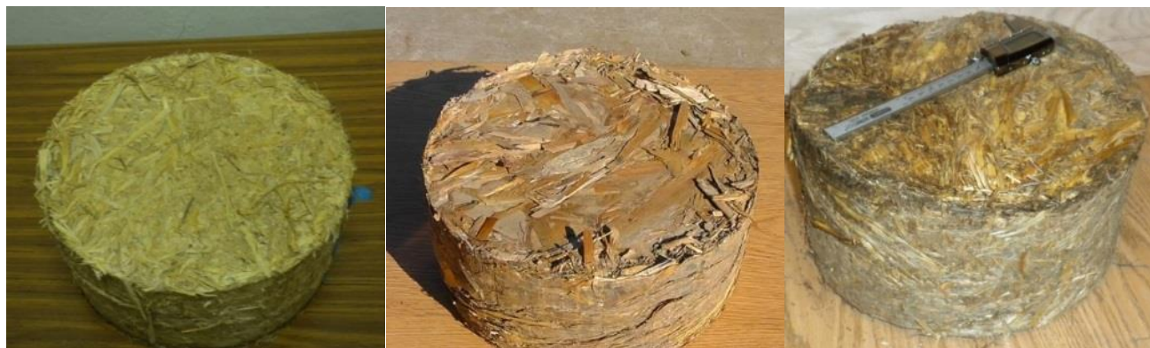
Figure 5: Densified Feedstock Logs; A) Switchgrass, B) Corn Stover, and C) Wheat Straw
