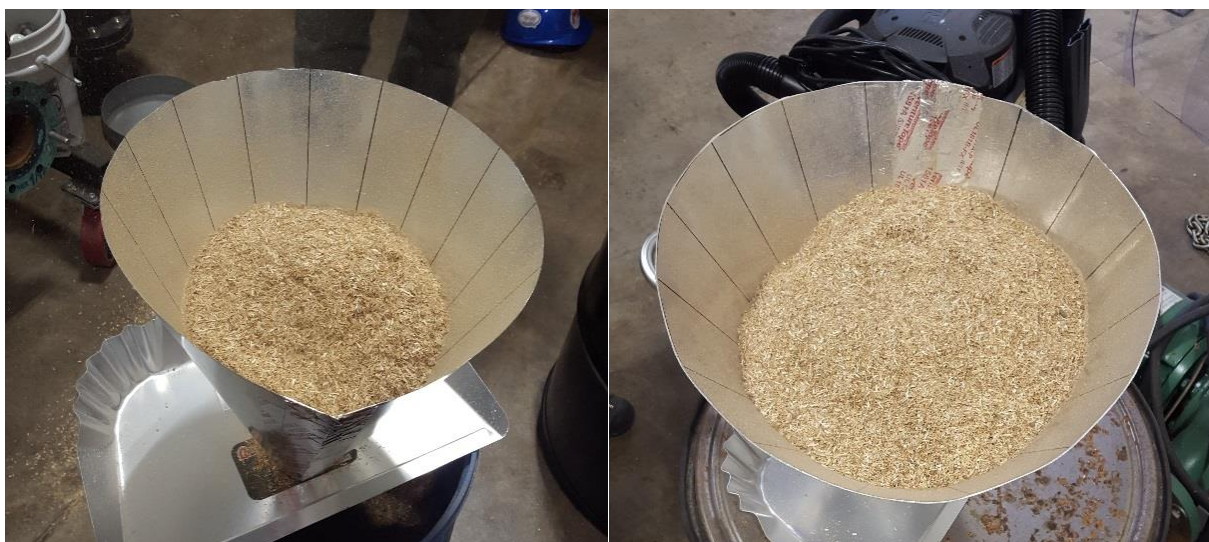
Figure 17: Test of Biomass Followability with 45-degree (Left) and 60-degree (Right) Cones
