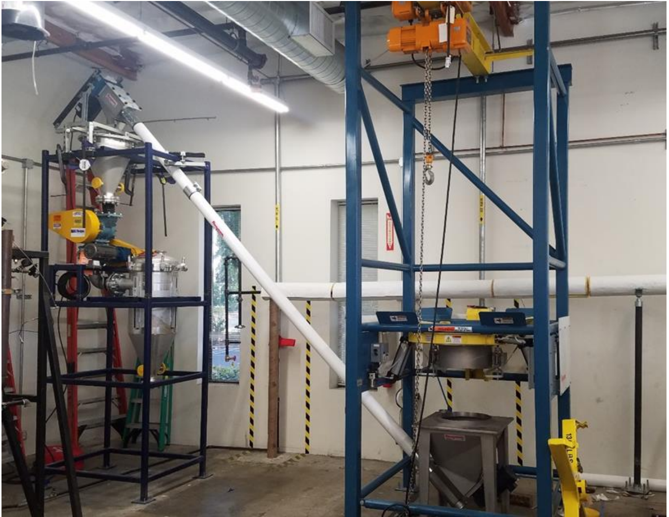
Figure 31: Completed Feed System Setup with Bulk-Bag Unloader
