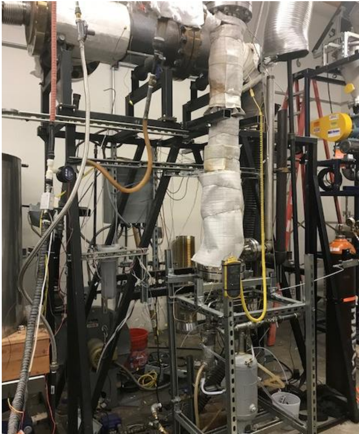
Figure 36: Installed Fuel Production Unit with Gasoline Condensers
