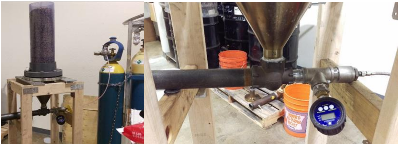
Figure 20: Feed Tests of Biomass for BCSGS Using a Test Set-up Consisting of Educator and Feed Purge Separator from Cost-Shared U.S. DOE Project
