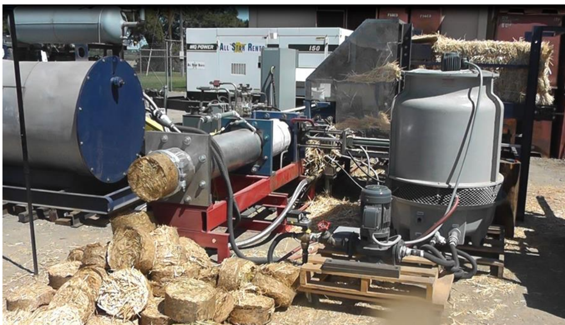
Figure 4: The Biomass Densification Equipment in BCSGS Full-Scale Plant for Densifying the Feedstocks to Minimize Feedstock Transportation Cost and Energy
