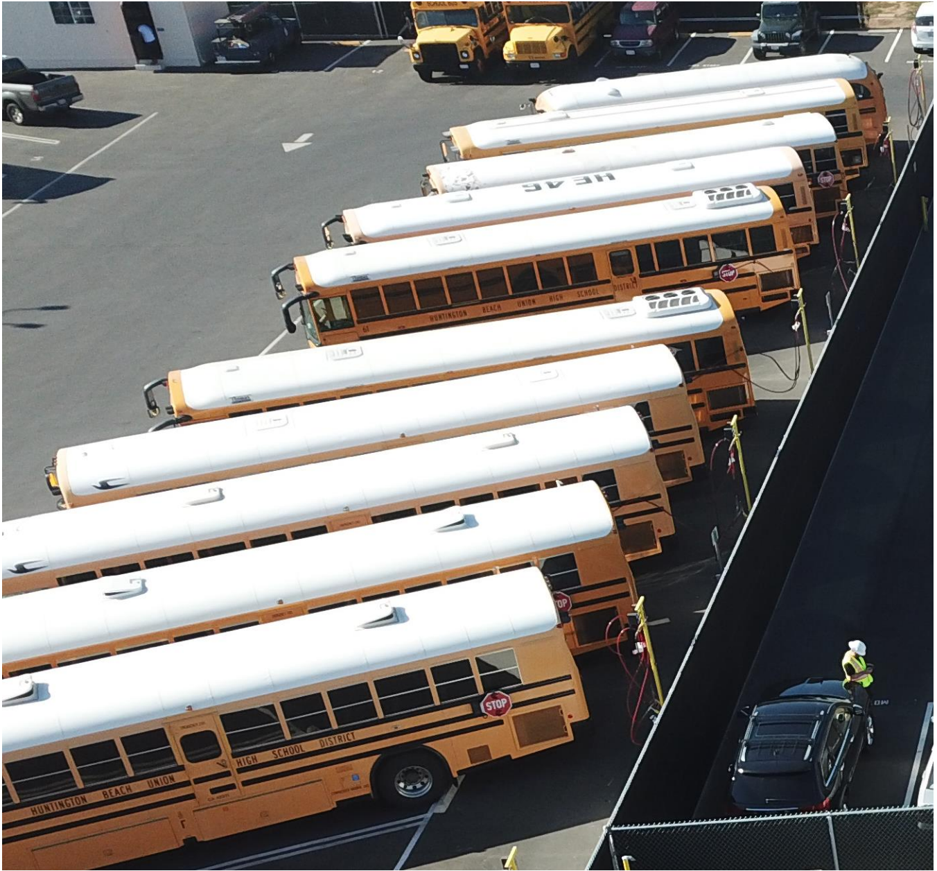
Figure 2: HBUHSD Buses Refueling Using Time-Fill Posts
