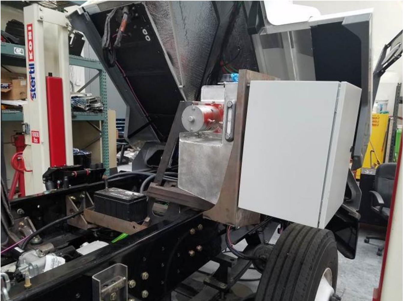
Figure 17: Test Fitting of First PCAS into Tractor #1
