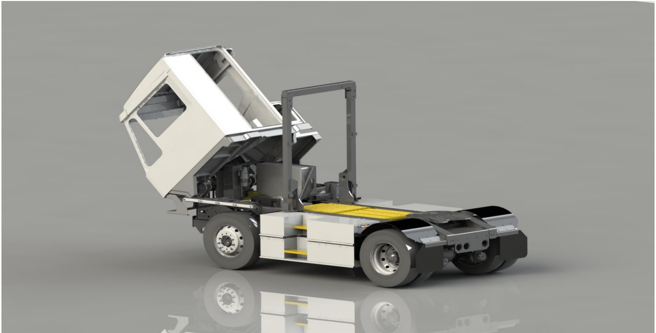
Figure 12: Illustration of T2 with Drive System Installed
