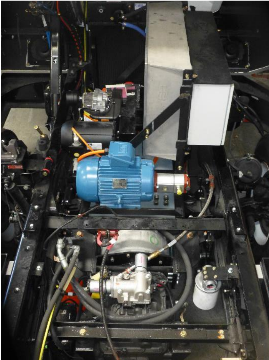
Figure 6: Gen-2 PCAS and MDS Installed in the Tractor
