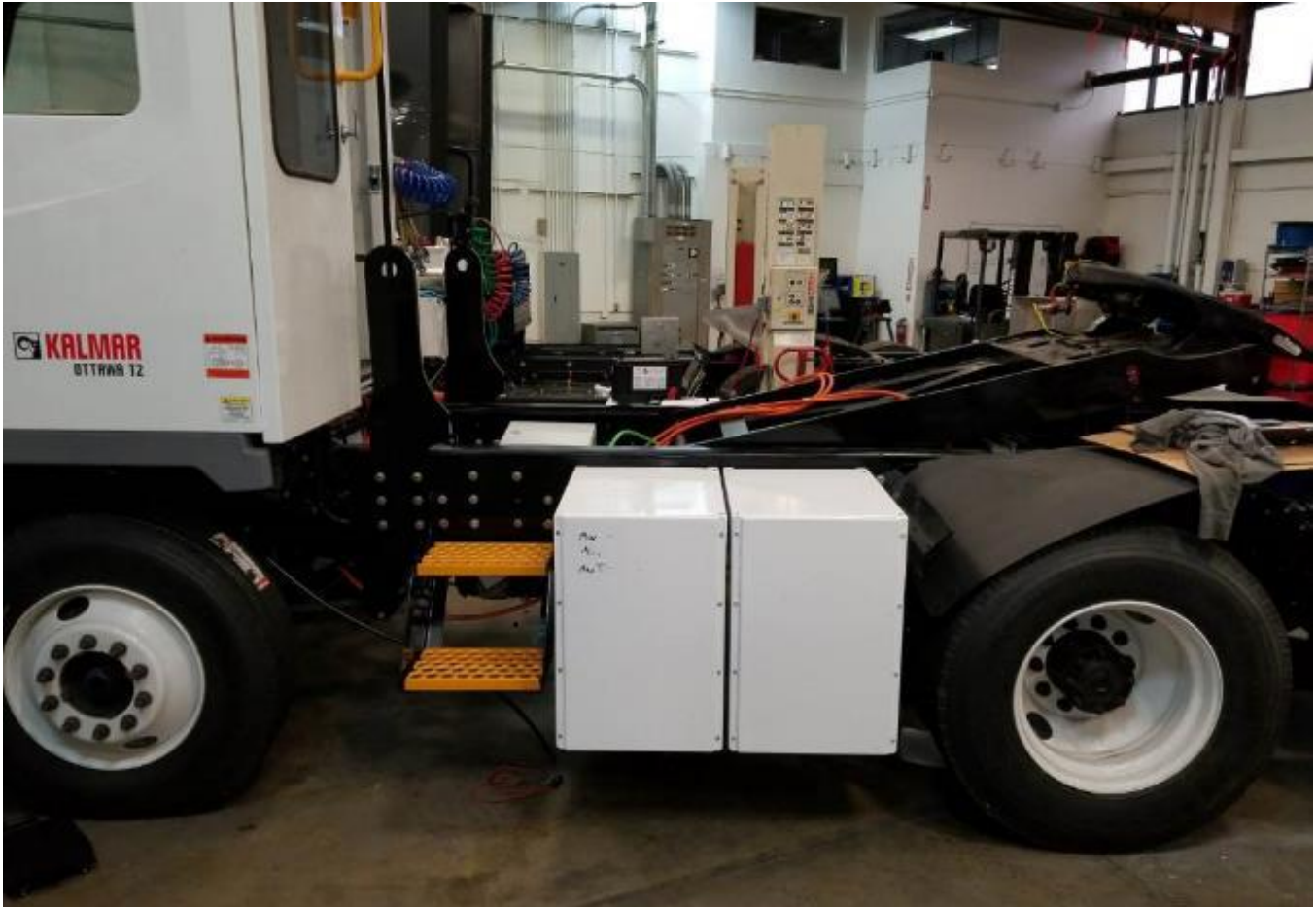
Figure 24: Tractor #4 Built for IKEA with Nissan Battery Enclosures
