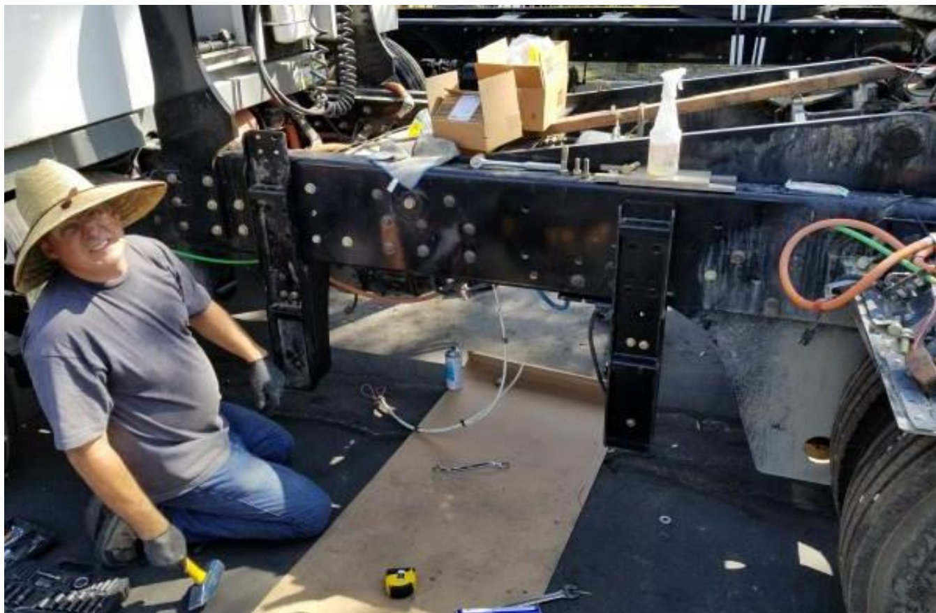
Figure 23: Tractor #1 Having Its ESS Mounts Replaced, August 2017
