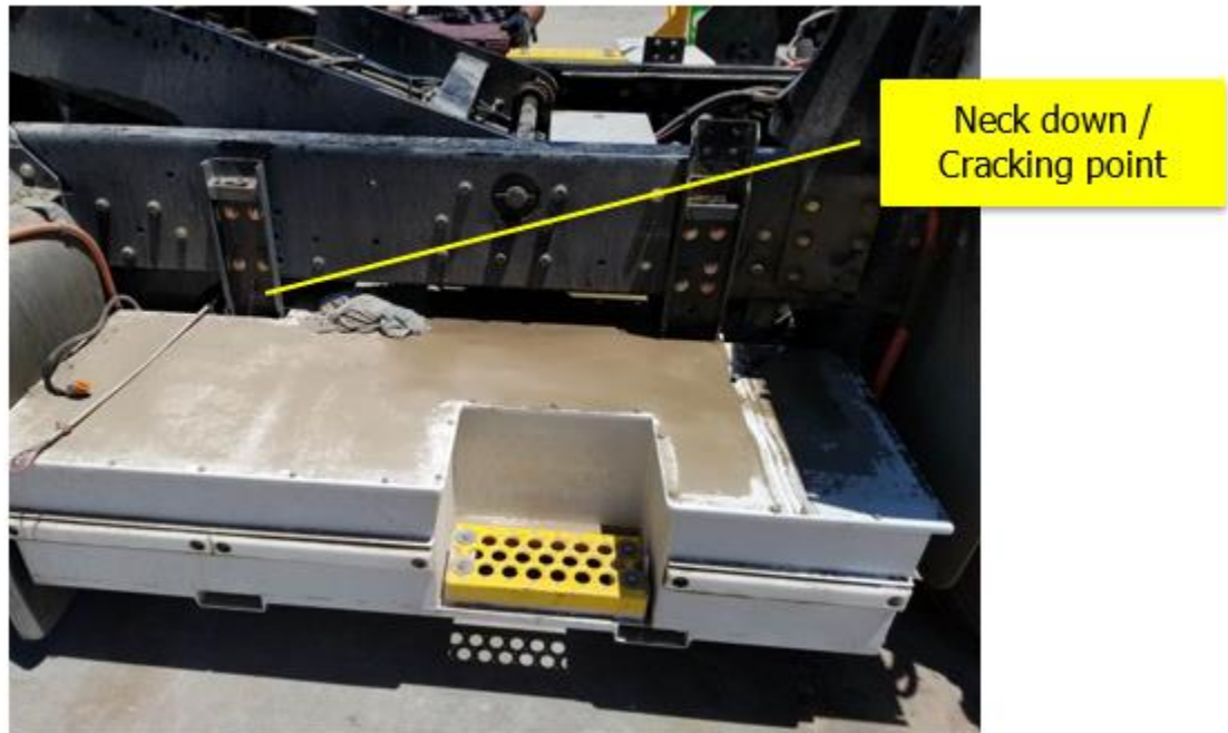
Figure 29: Grimmway's Tractor with Upper ESS Box Removed
