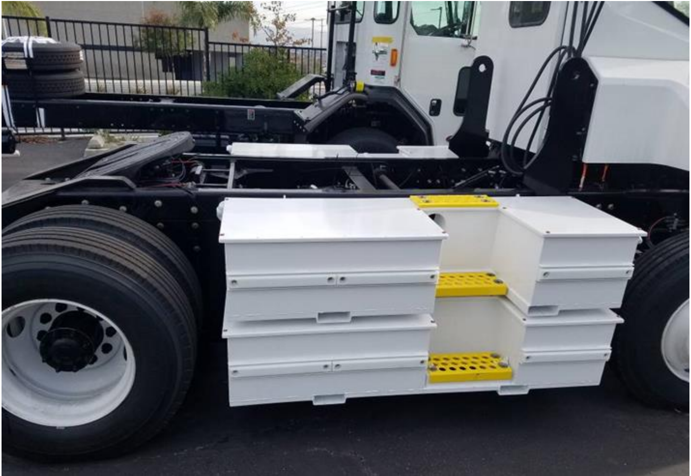
Figure 19: ESS Enclosures Mounted to Side of Tractor #1
