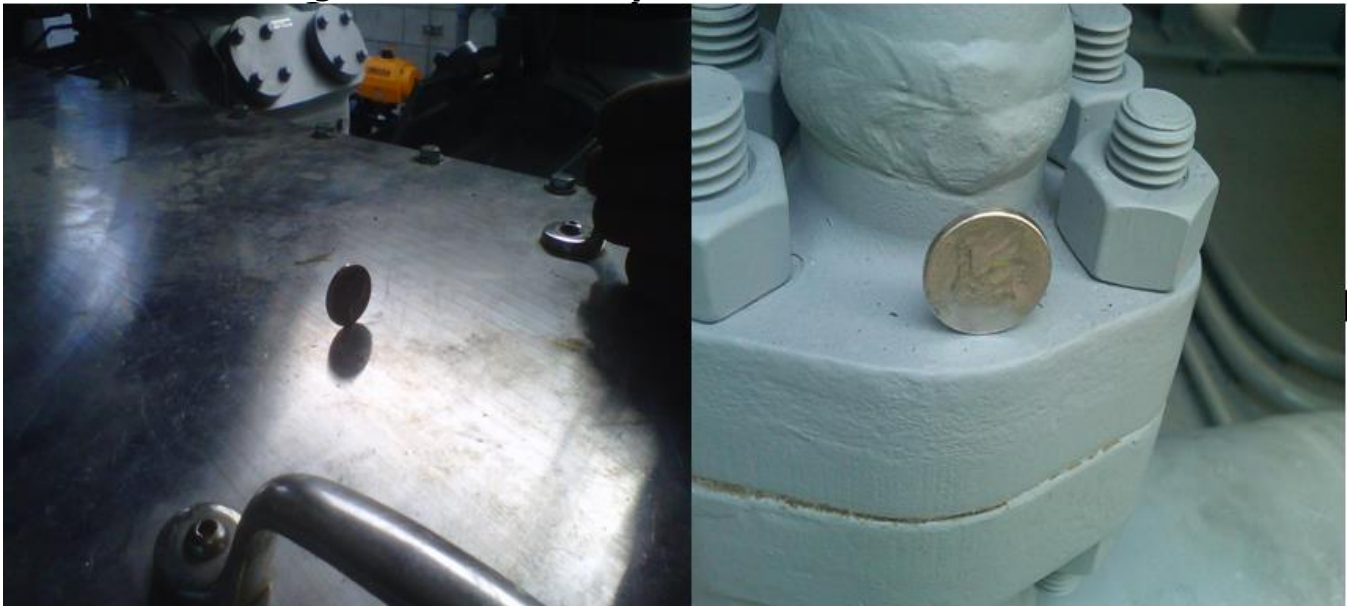
Figure 4: Substantially Reduced Vibration Levels
