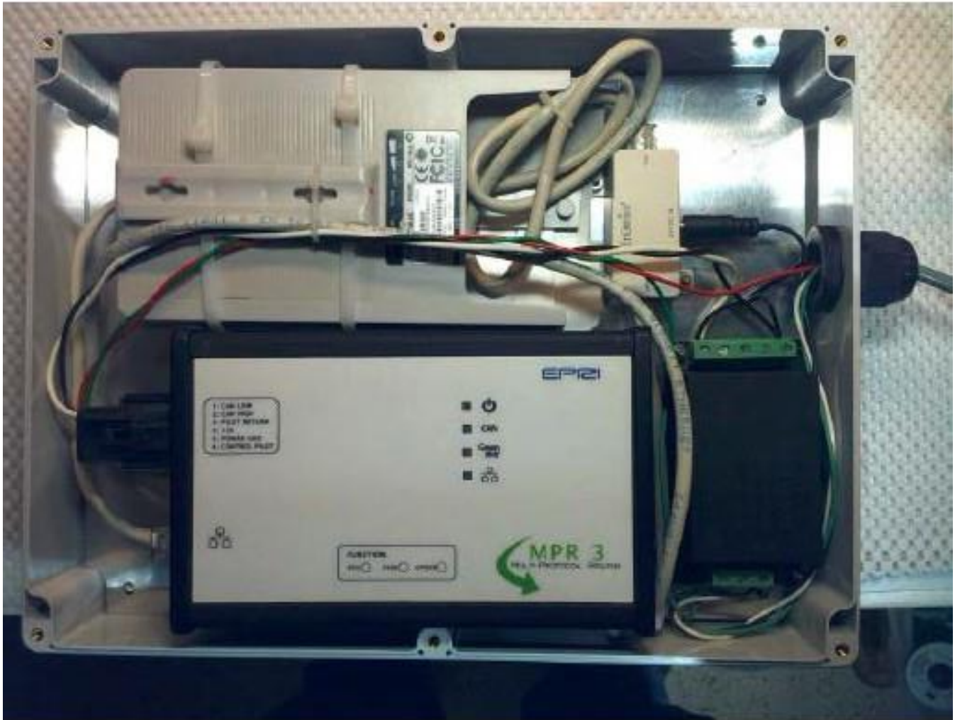
Figure 121: EVSE Communication Box Layout and Contents
