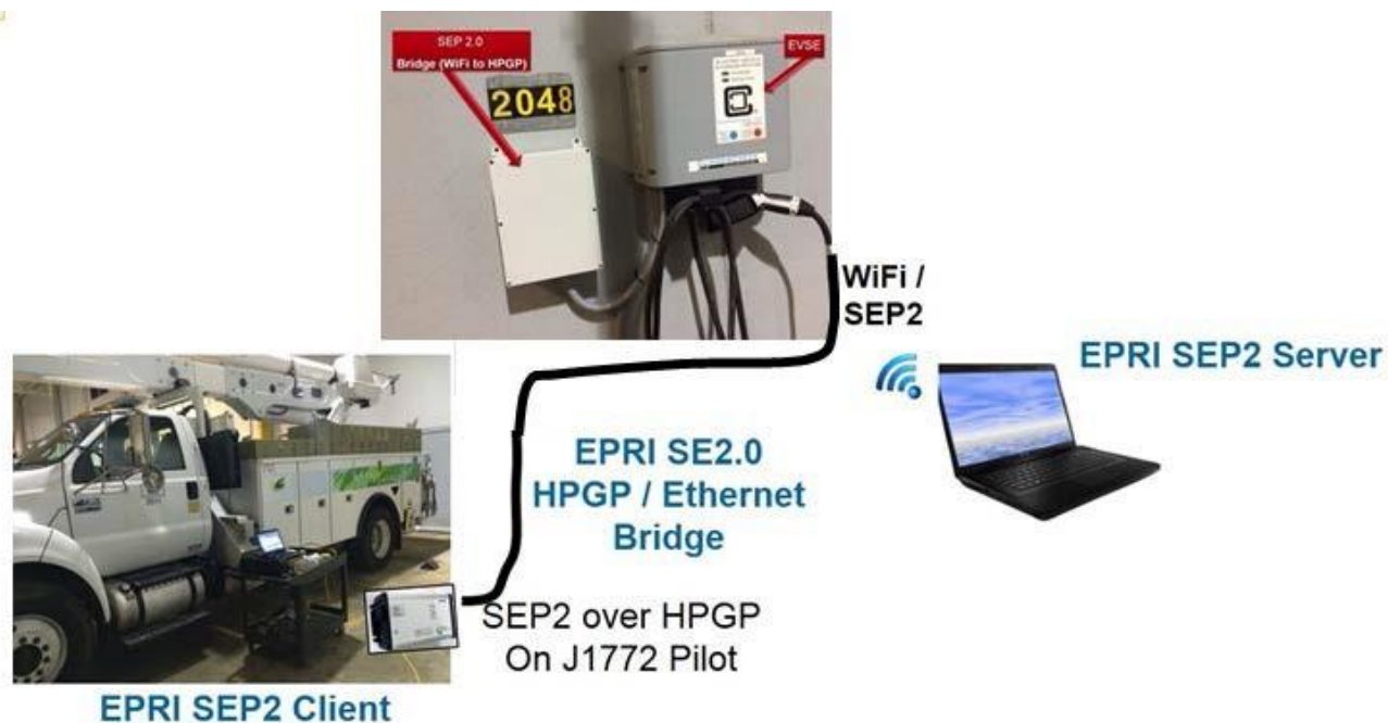
Figure 122: Smart Charging Setup and Layout at the Knoxville Utility Board
