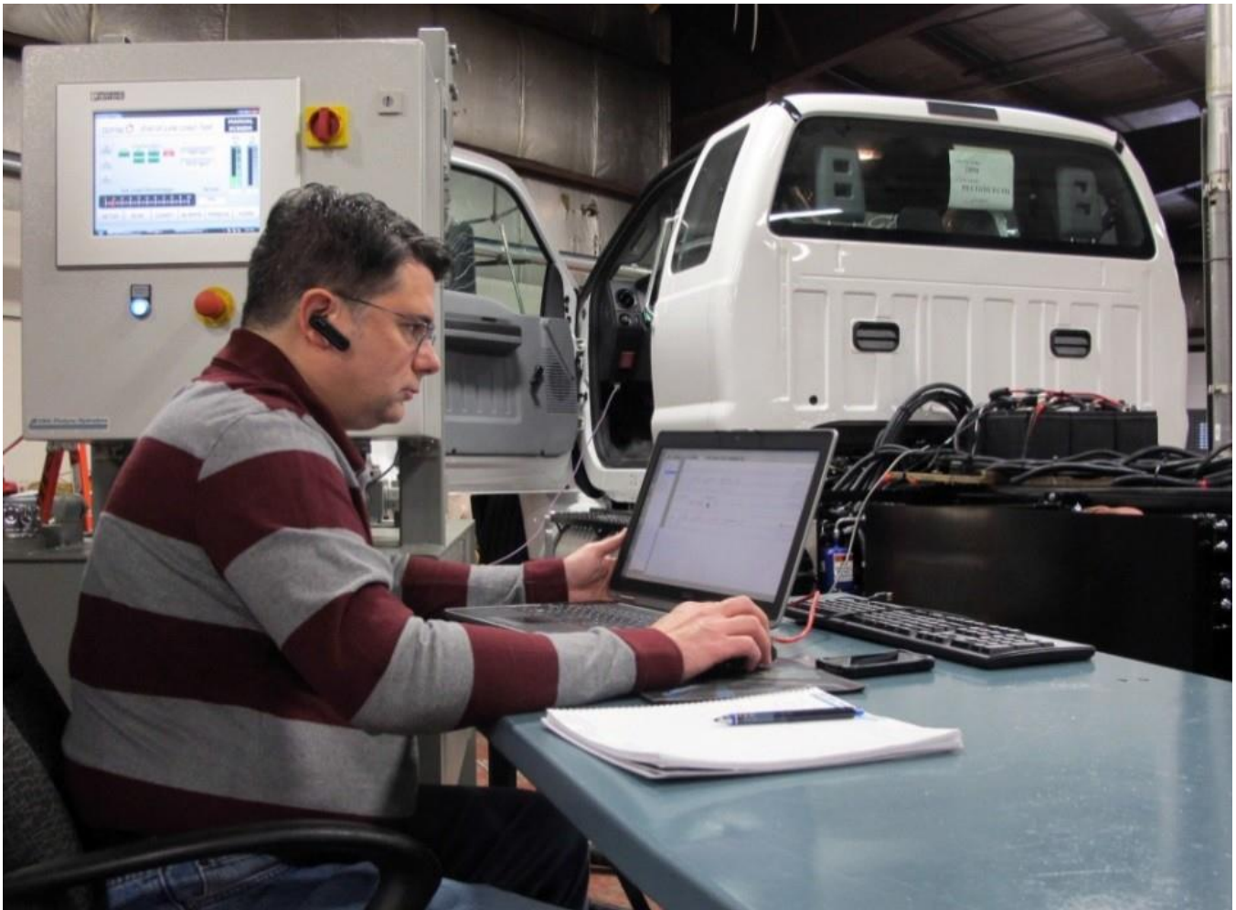
Figure 27: Using the Automatic Tester for Testing the Final Assembled Hybrid System
