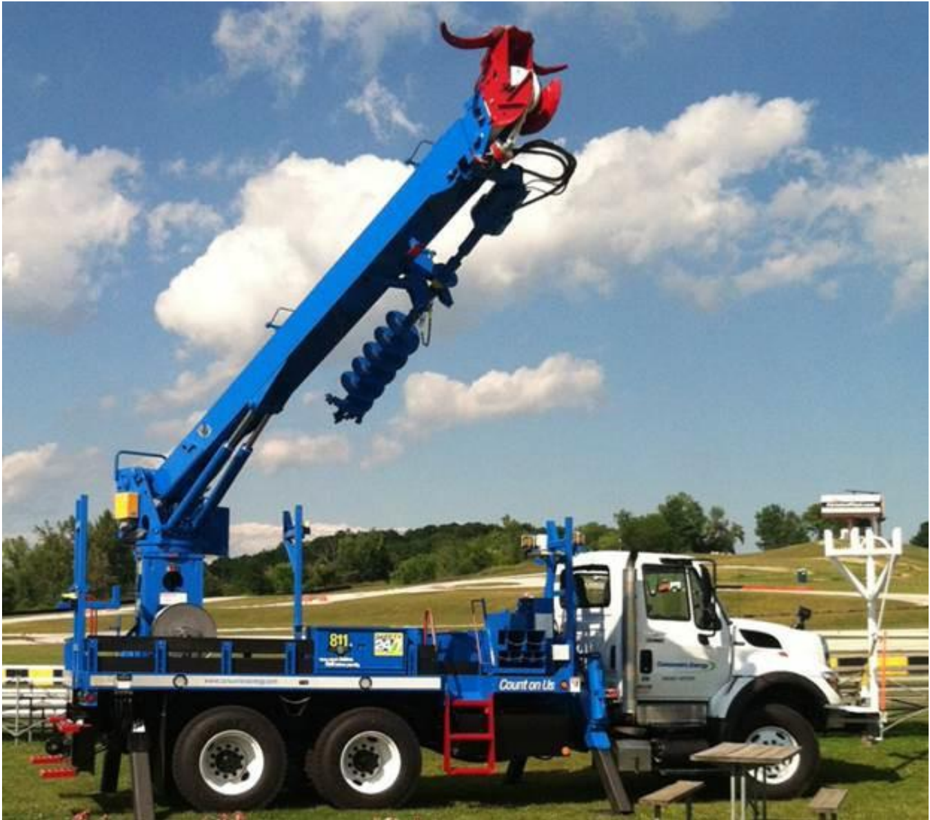
Figure 23: Final Configuration as a Digger Derrick
