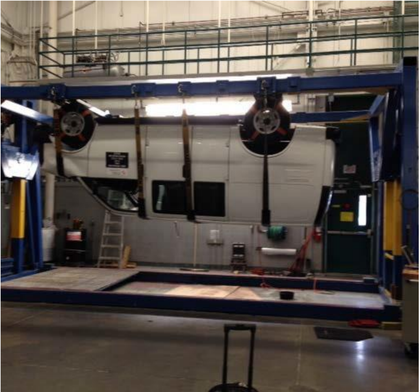
Figure 89: Van Rollover Test
