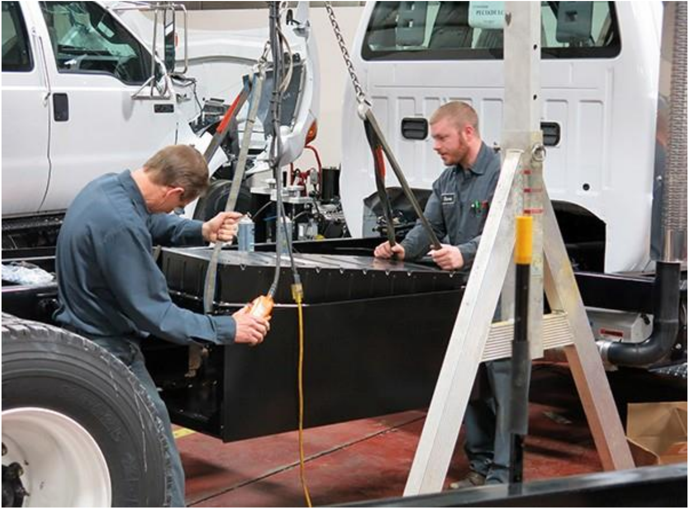
Figure 26: Installing a Battery onto a Chassis
