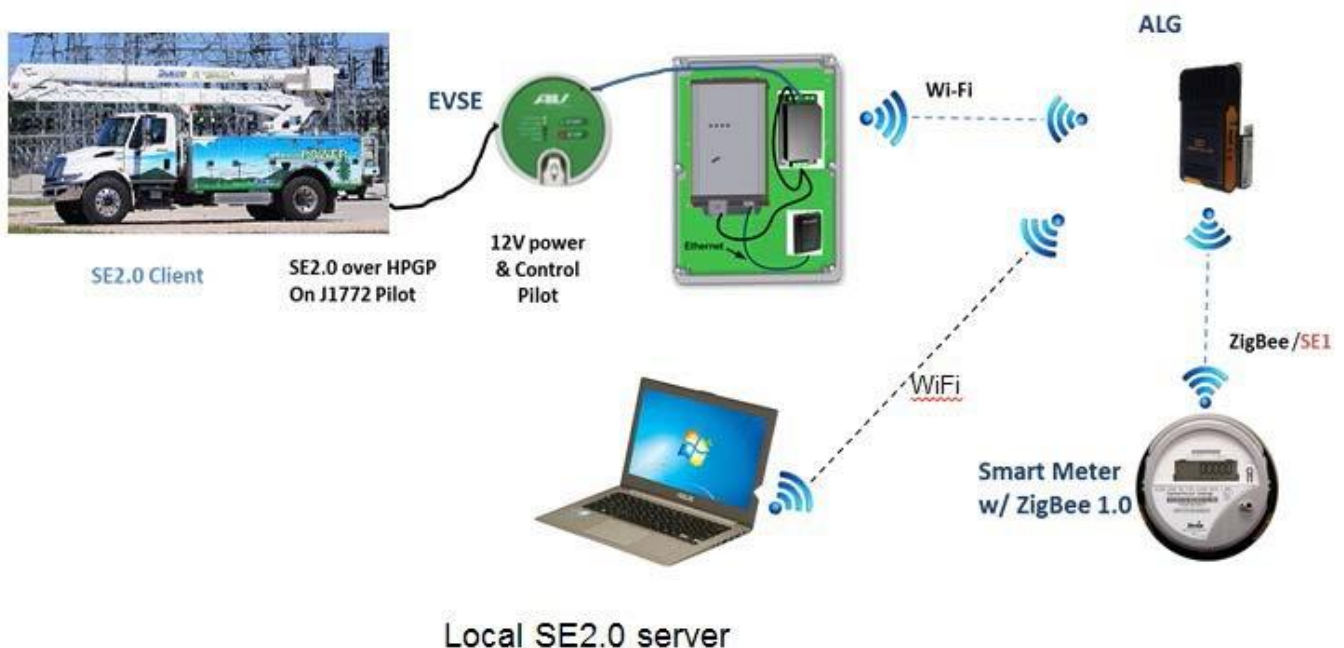
Figure 115: Single Plug-In Vehicle Communication Architecture
