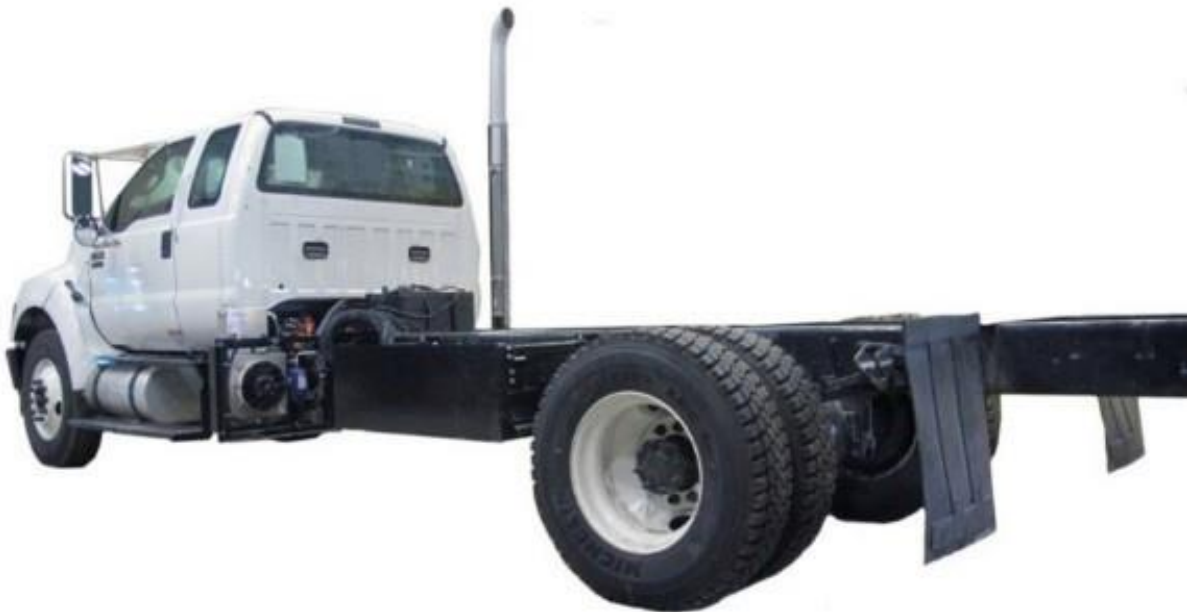
Figure 22: Chassis with Hybrid System Installed
