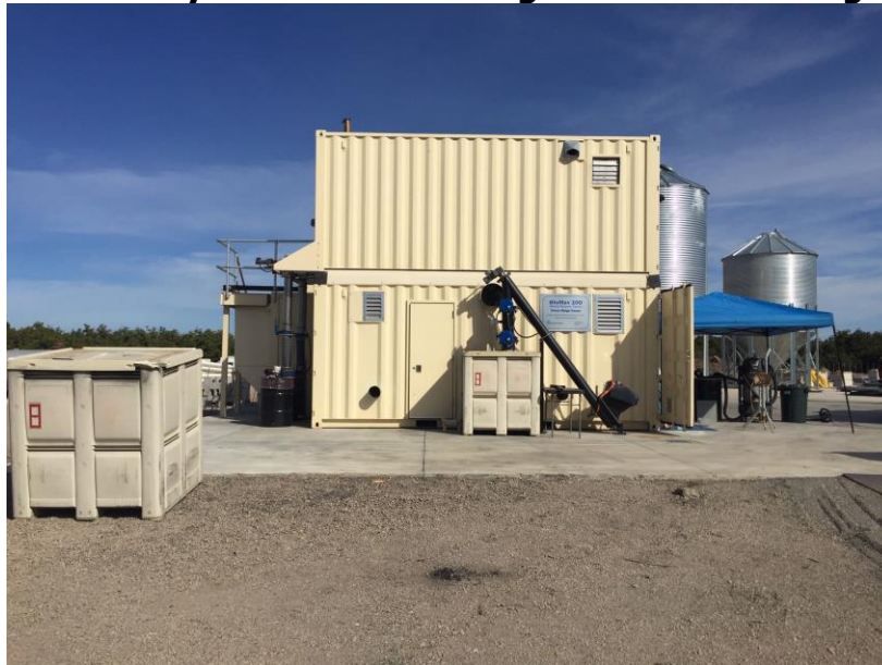
Figure 19: Gasification System at Dixon Ridge Farms Producing Walnut Biochar
