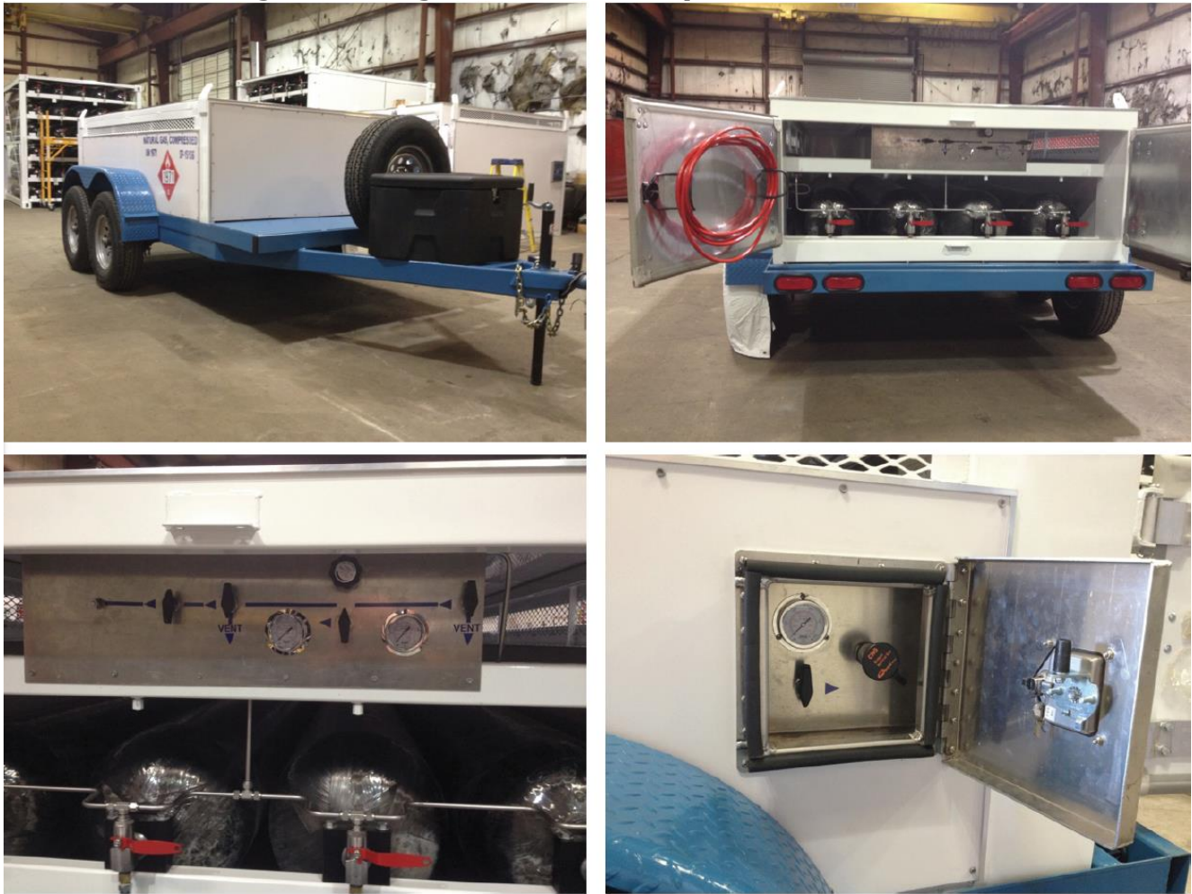
Figure 23: High-Pressure Gas Cylinder Tube Trailer
