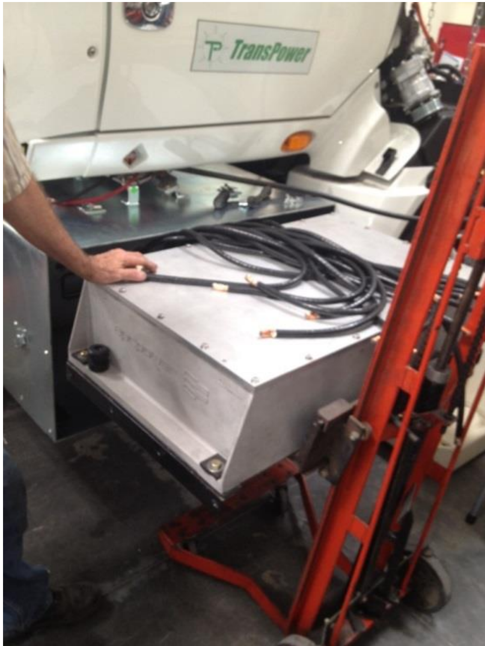
Figure 26: ICU Being Installed into Truck #2
