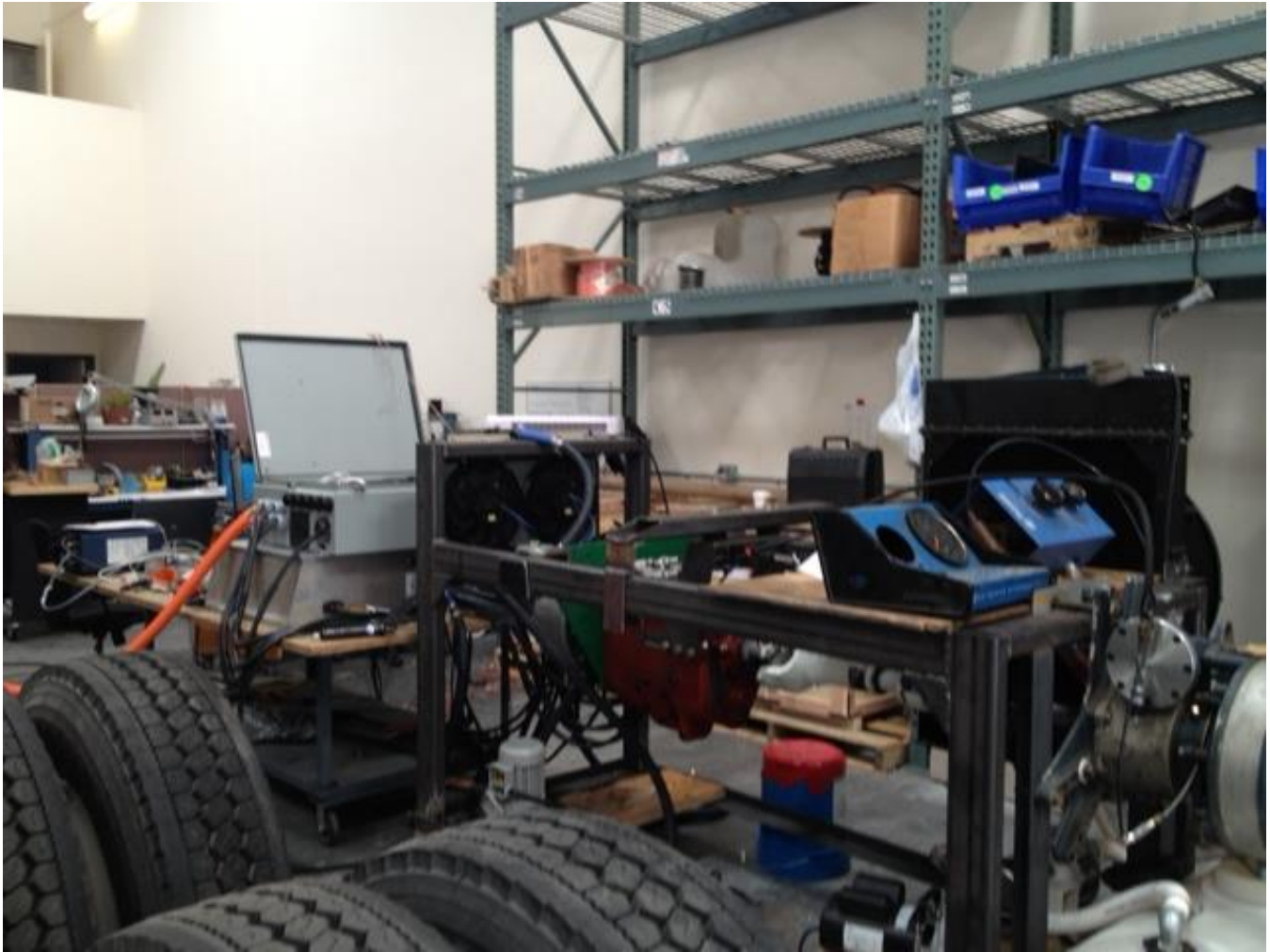
Figure 4: Complete Dynamometer Assembly Showing Fisker Motor, AMT, and Dynamometer Water Brake Mechanism
