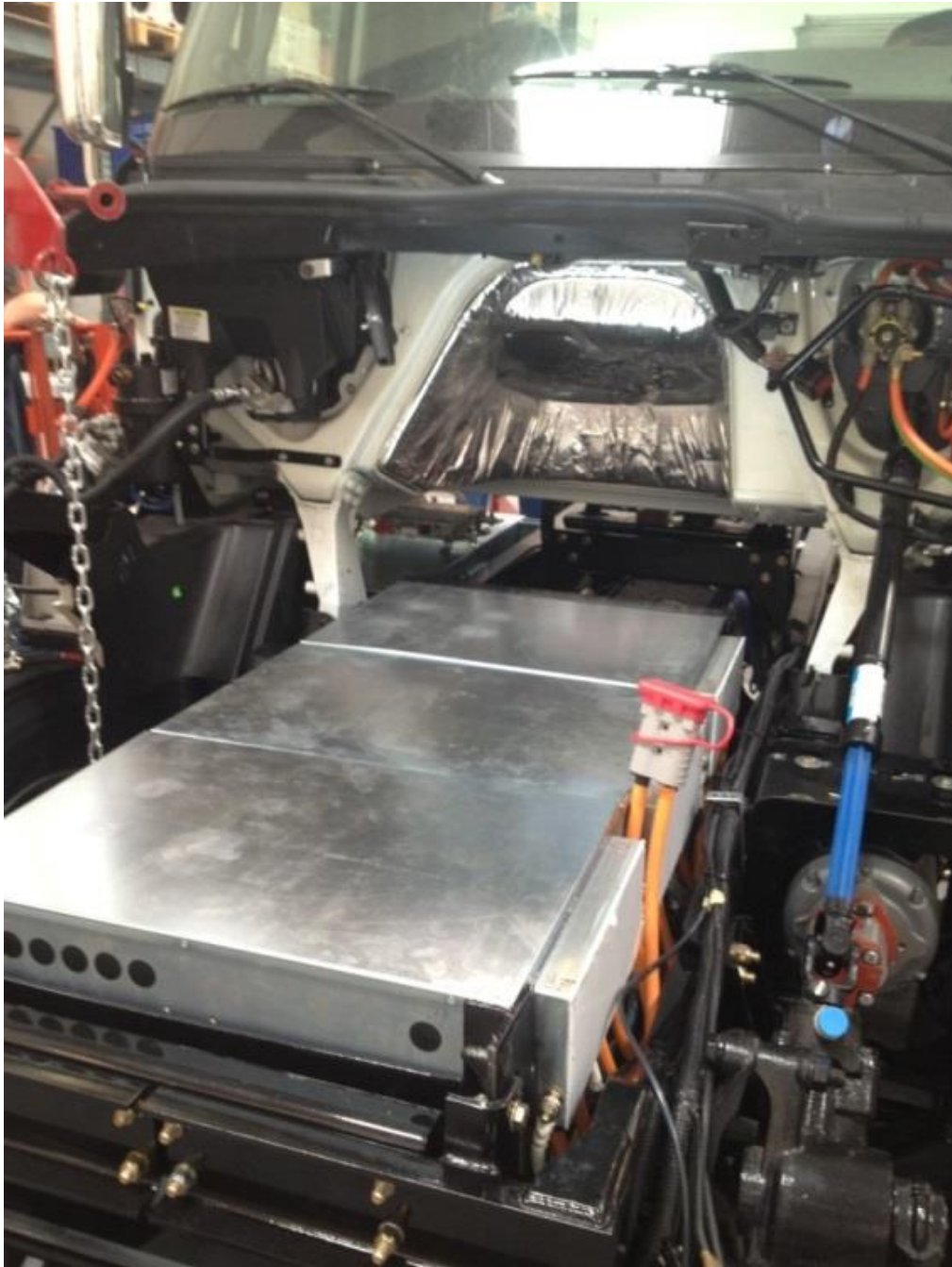
Figure 25: ESS Mile-Max™ Modules Installed in Engine Compartment of Truck #2
