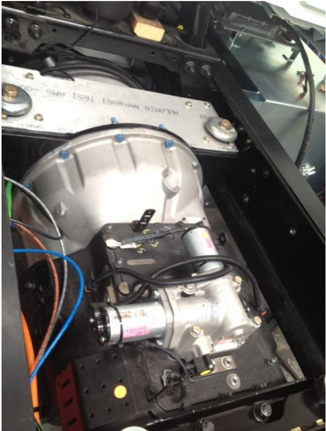
Figure 24: Motor-Transmission Assembly after Installation into Truck #2
