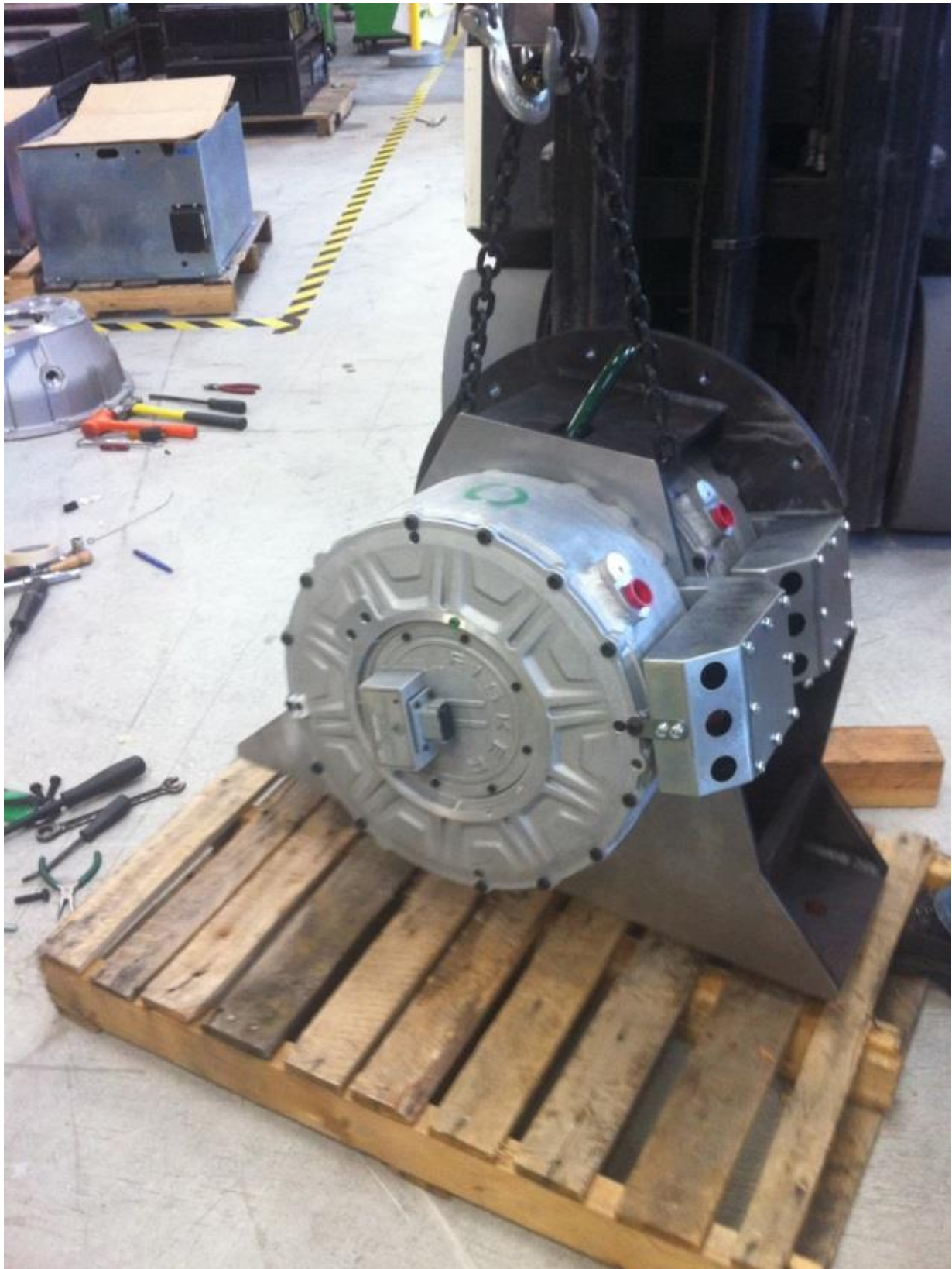
Figure 19: Completed Drive Motors after Integration into Dual Motor Support Structure
