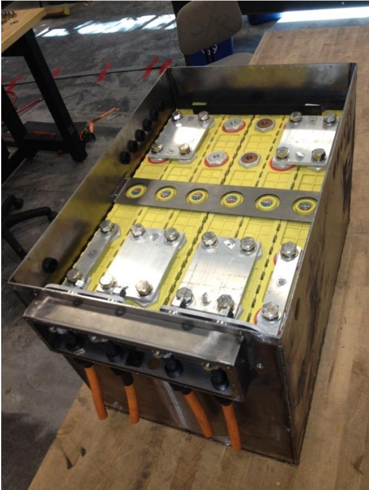
Figure 2: Mile-Max™ Module Using 700 Ah Lithium-Ion Battery Cells
