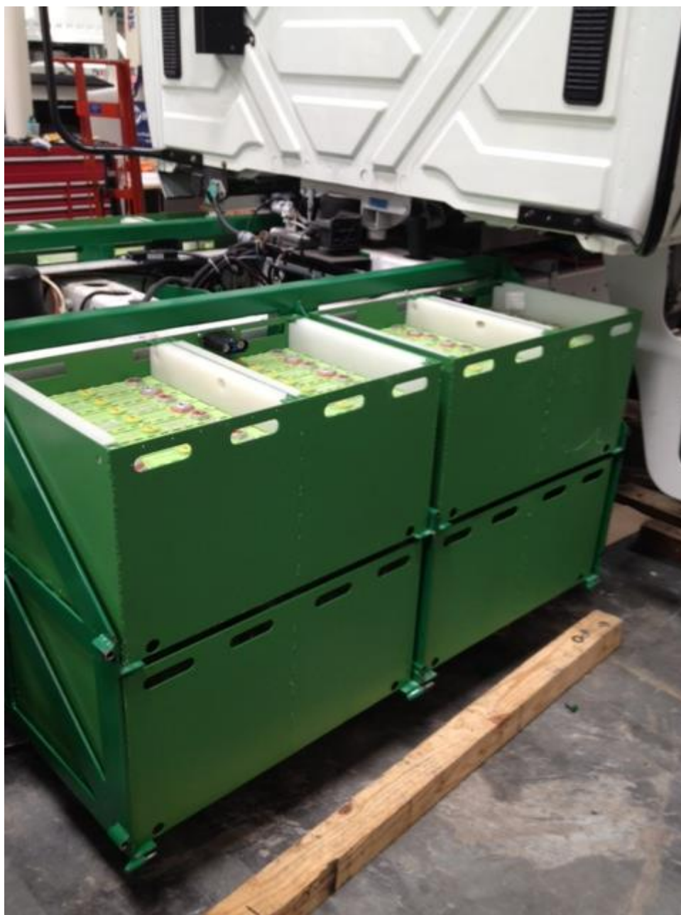
Figure 10: Updated Battery Module Design Incorporated into Truck #1
