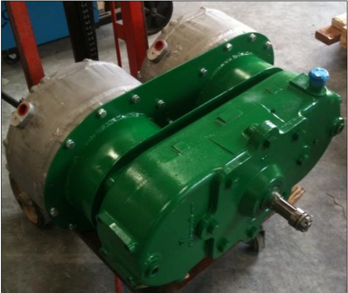
Figure 6: Original Main Propulsion Unit Developed for First Prototype
