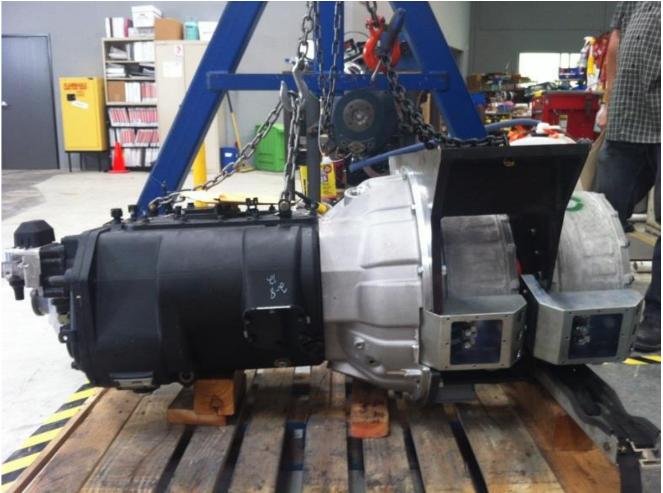
Figure 20: Dual Motor Assembly Mounted to 10-Speed Eaton Transmission
