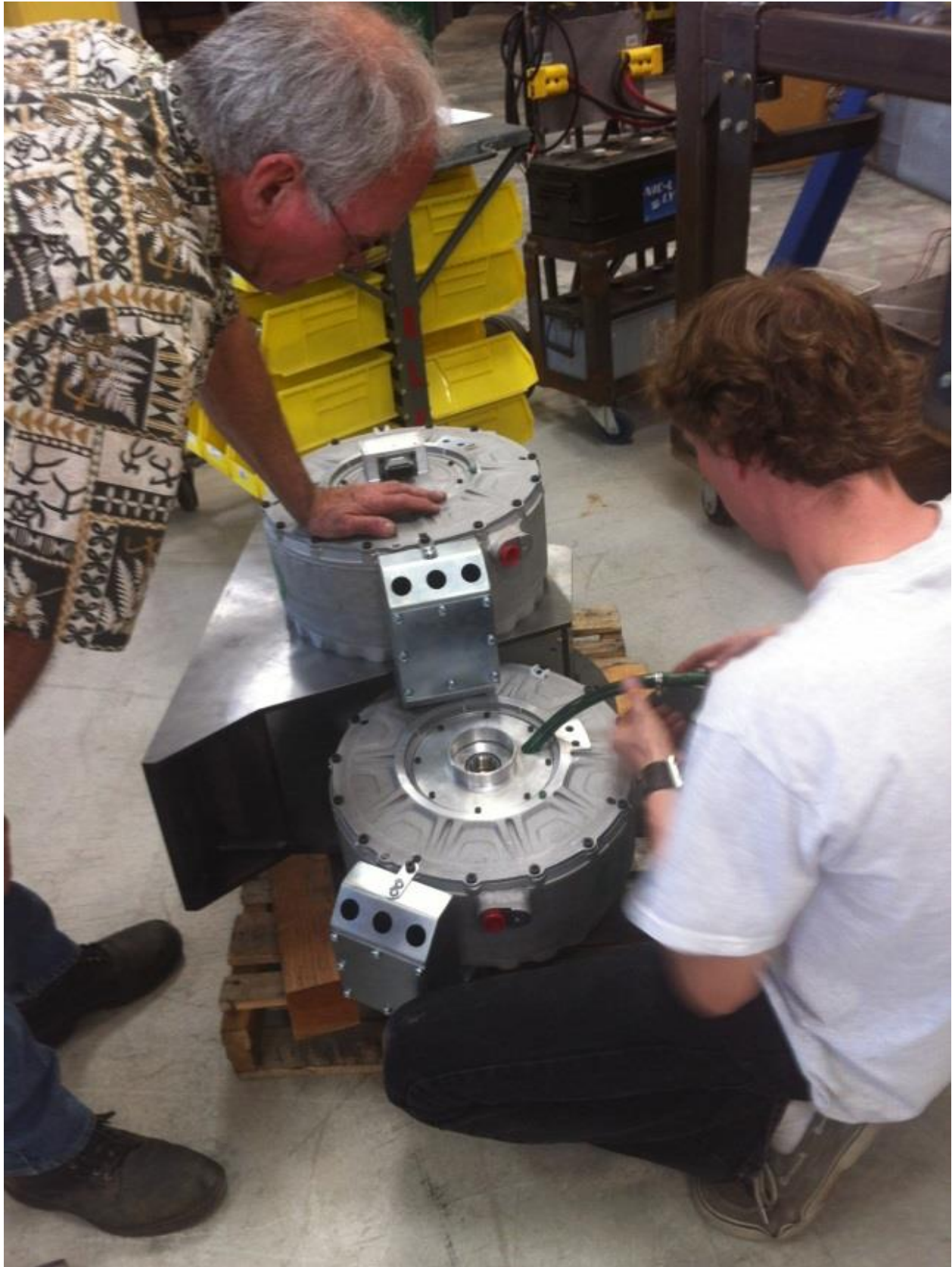
Figure 18: Drive Motors Installed in Dual Motor Support Structure
