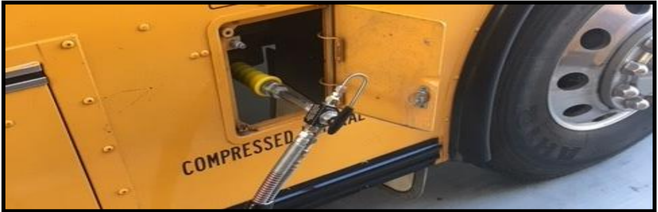
Figure 7: Bus Connected to Slow Fill Station
