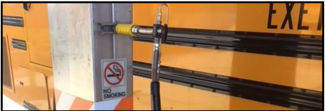
Figure 6: Filling Hose Attached to Pillar
