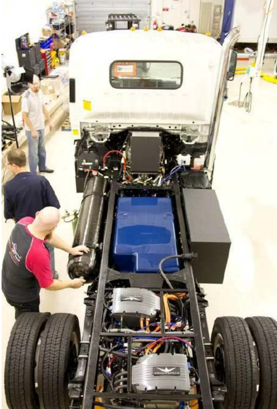
Figure 2: Wrightspeed Test Platform with Digital Drive System Installed
