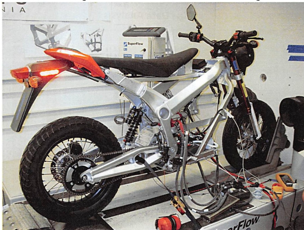
Figure 11: Chassis Dynamometer Run with AEVP Motorcycle Test Mule
