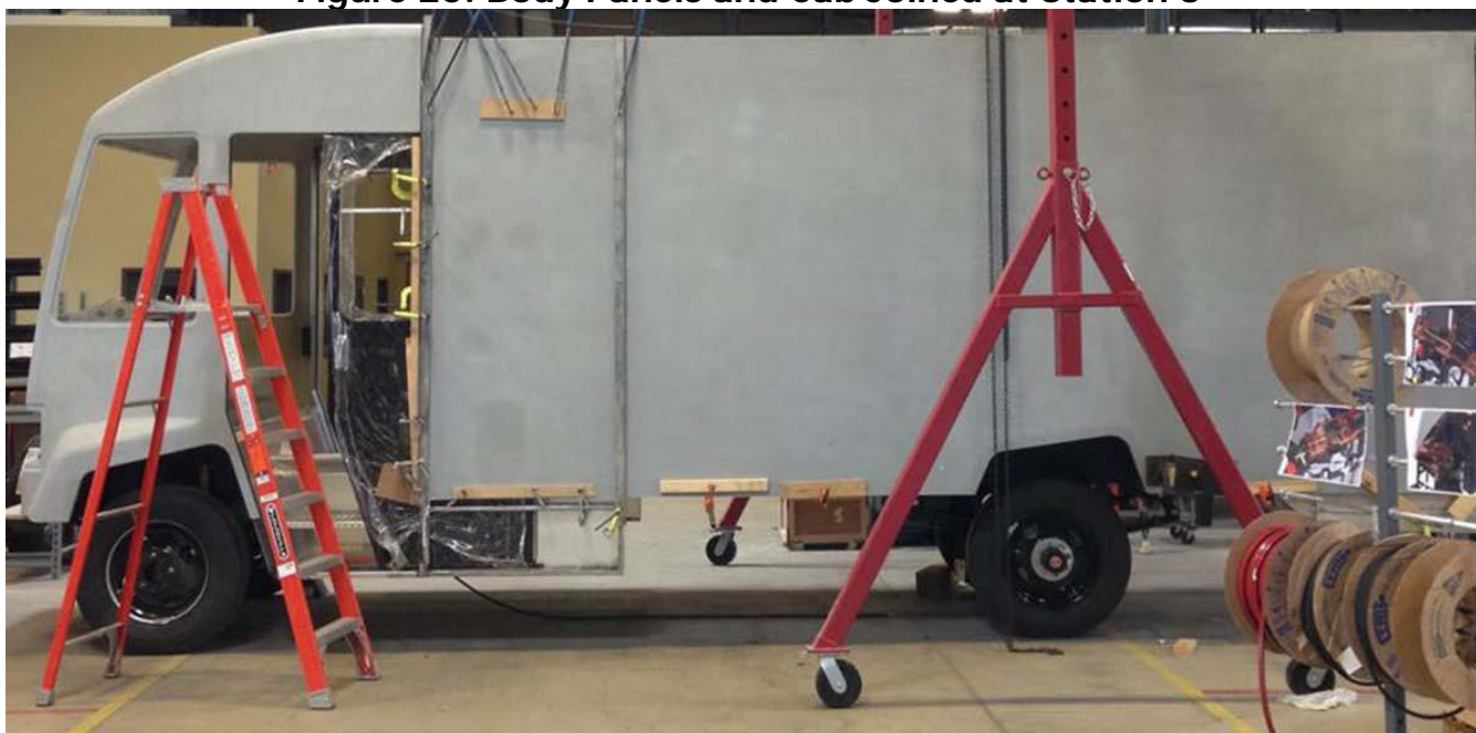
Figure 20: Body Panels and Cab Joined at Station 3
