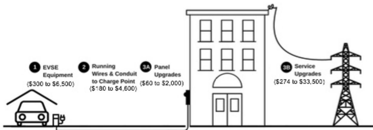
Figure 11: Potential Costs at the Different Stages of EVSE Installation at MUD Locations
