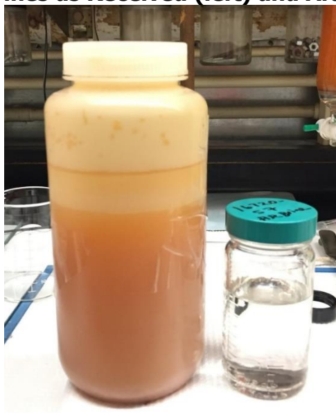
Figure 3: Geothermal Brines as Received (left) and After Pre-treatment (right)
