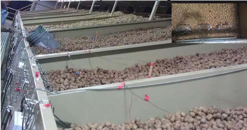
Figure 17: Experimental Setup of Hot Air Drying of IR Predried Walnuts
