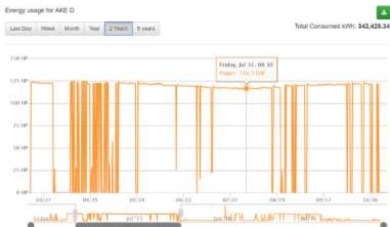
Figure 32: Drop in Power Level During the Season as the Water Table is Falling
