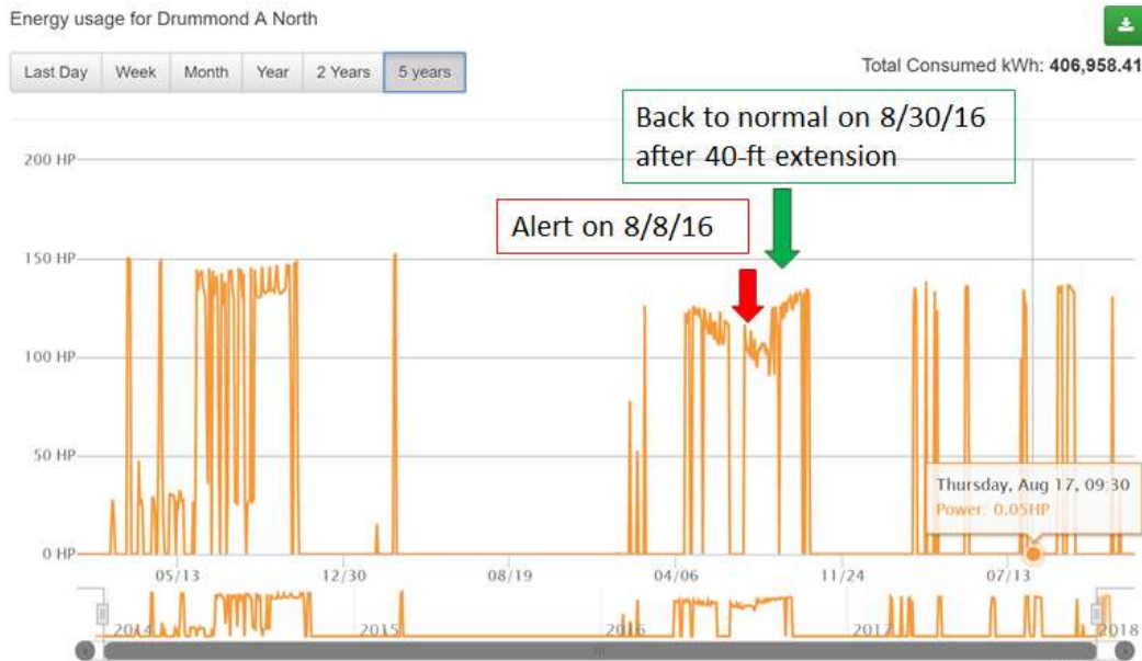
Figure 83: Smart Meter Data in 2014 to 2017 for Well Pump Drummond A North
