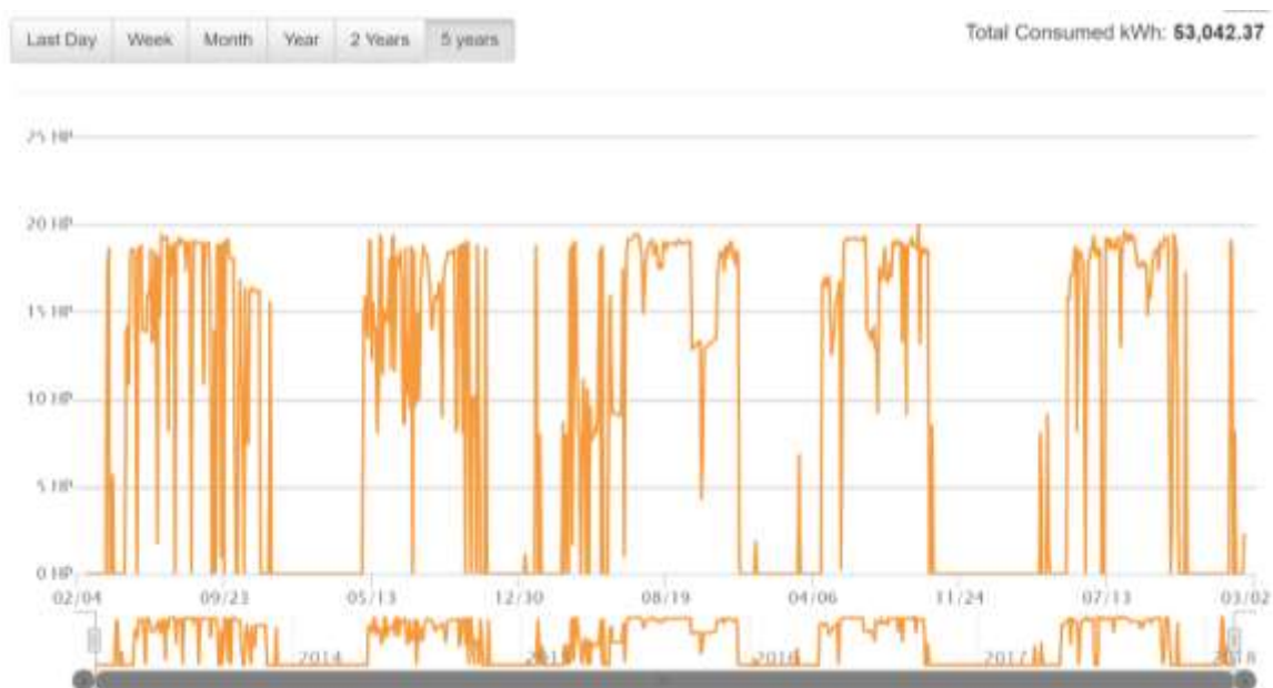
Figure 122: History of Energy Use of the Irrigation Pump at a Ranch from 2013 to 2018
