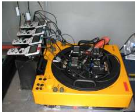
Figure 42: Camera System Mounted in the Belly of the Aircraft
