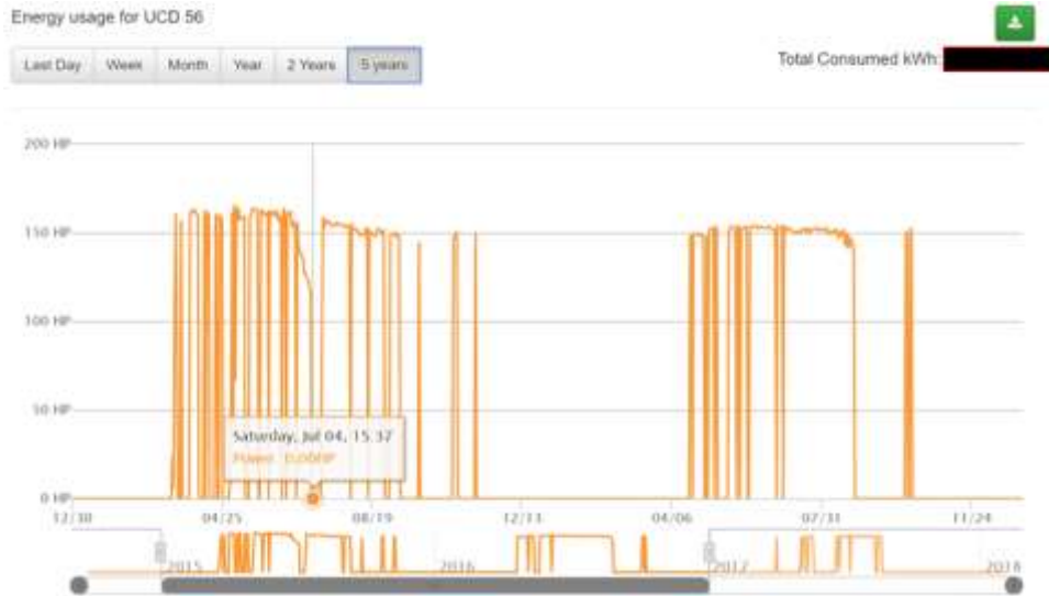
Figure 97: Smart Meter Data from the Well Pump at Site #4
