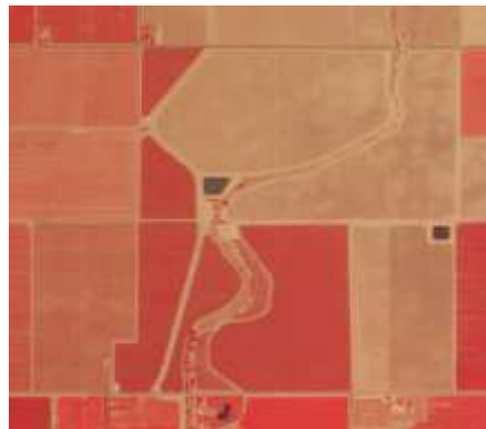
Figure 44: NIR, Red, Green Channels Combined Into Single Color Image
