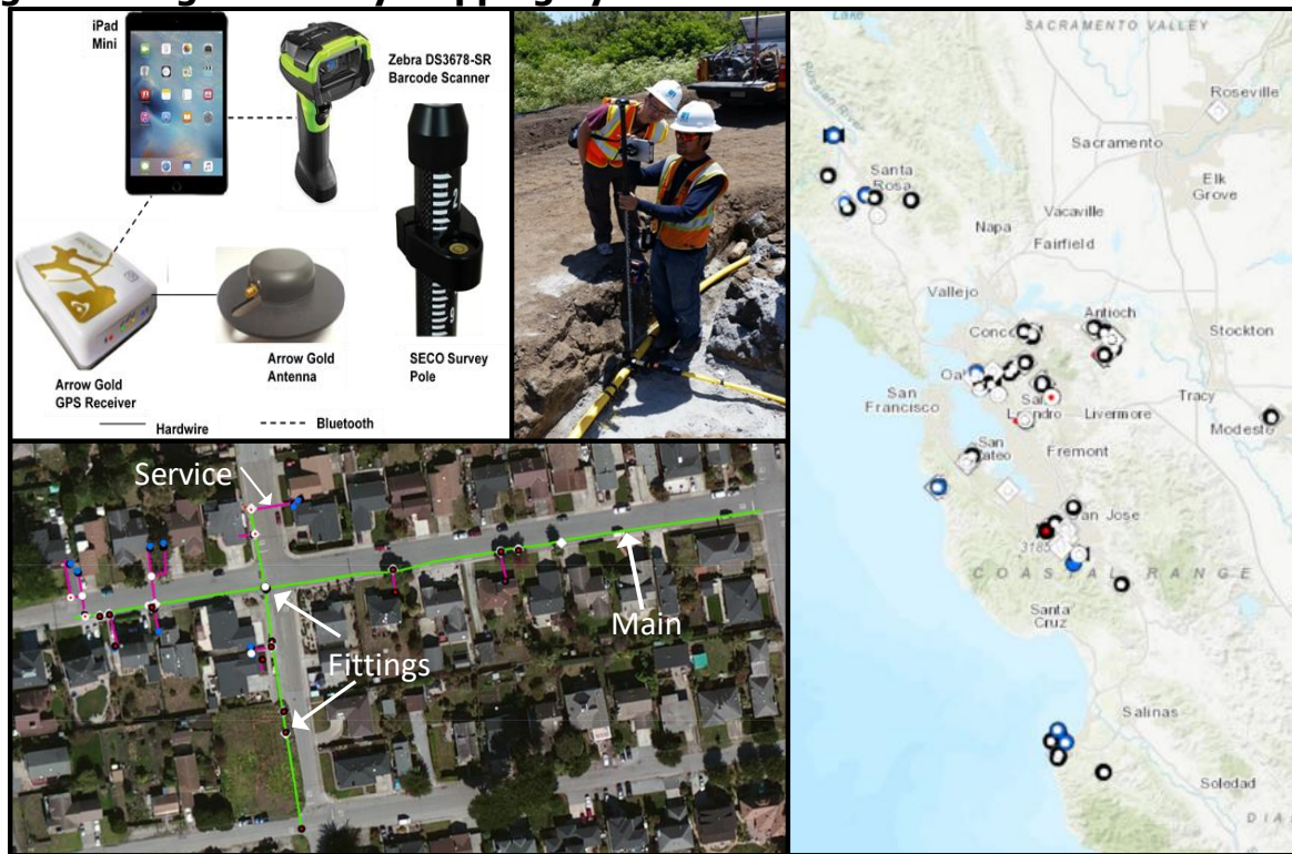
Figure 3: High Accuracy Mapping System – Hardware and Software Interface
