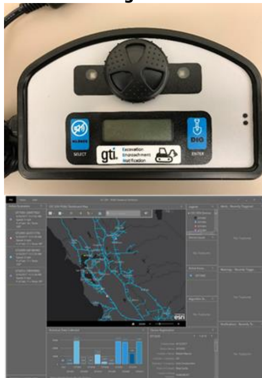
Figure 2: Global Positioning System Device on Excavator and Utility Monitoring Dashboard
