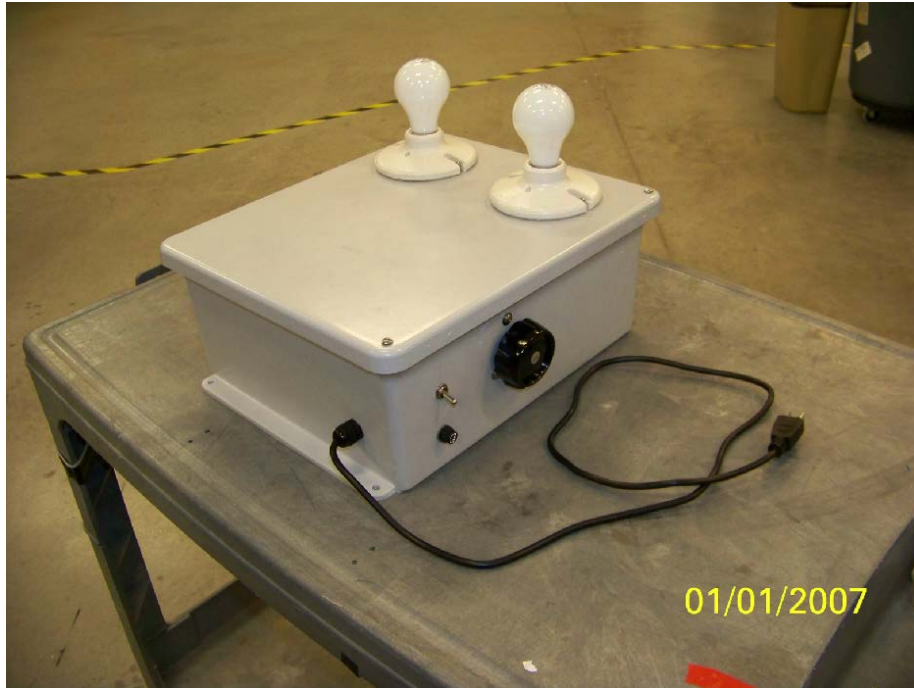
Figure 6: Transformer Emulator with Phantom Loading
