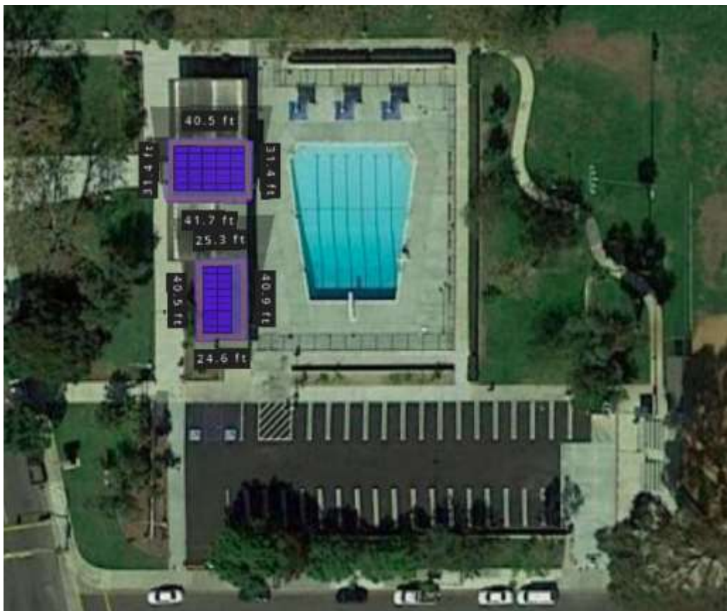
Figure A-12: Carson Park Pool (25KW PV, 2 Level II EVSE, 0 Battery)
