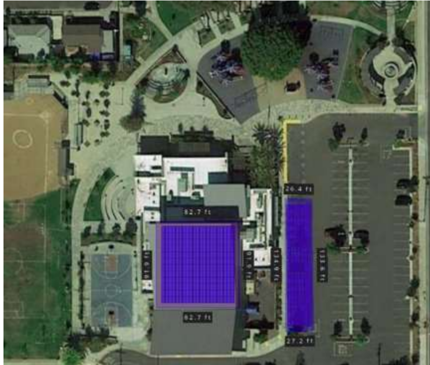
Figure A-14: Carson Park (160KW PV, 1044KWH/520KW Batteries, 2 Level II EVSE)
