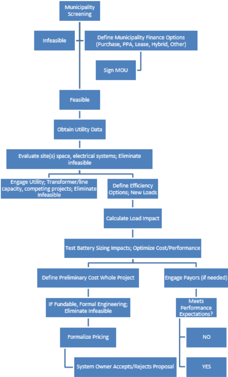
Figure 6: Process Diagram for Advanced Energy Community Design
