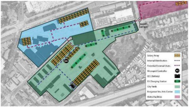
Figure 25: Potential Location for Microgrid Equipment and Distribution Routes
