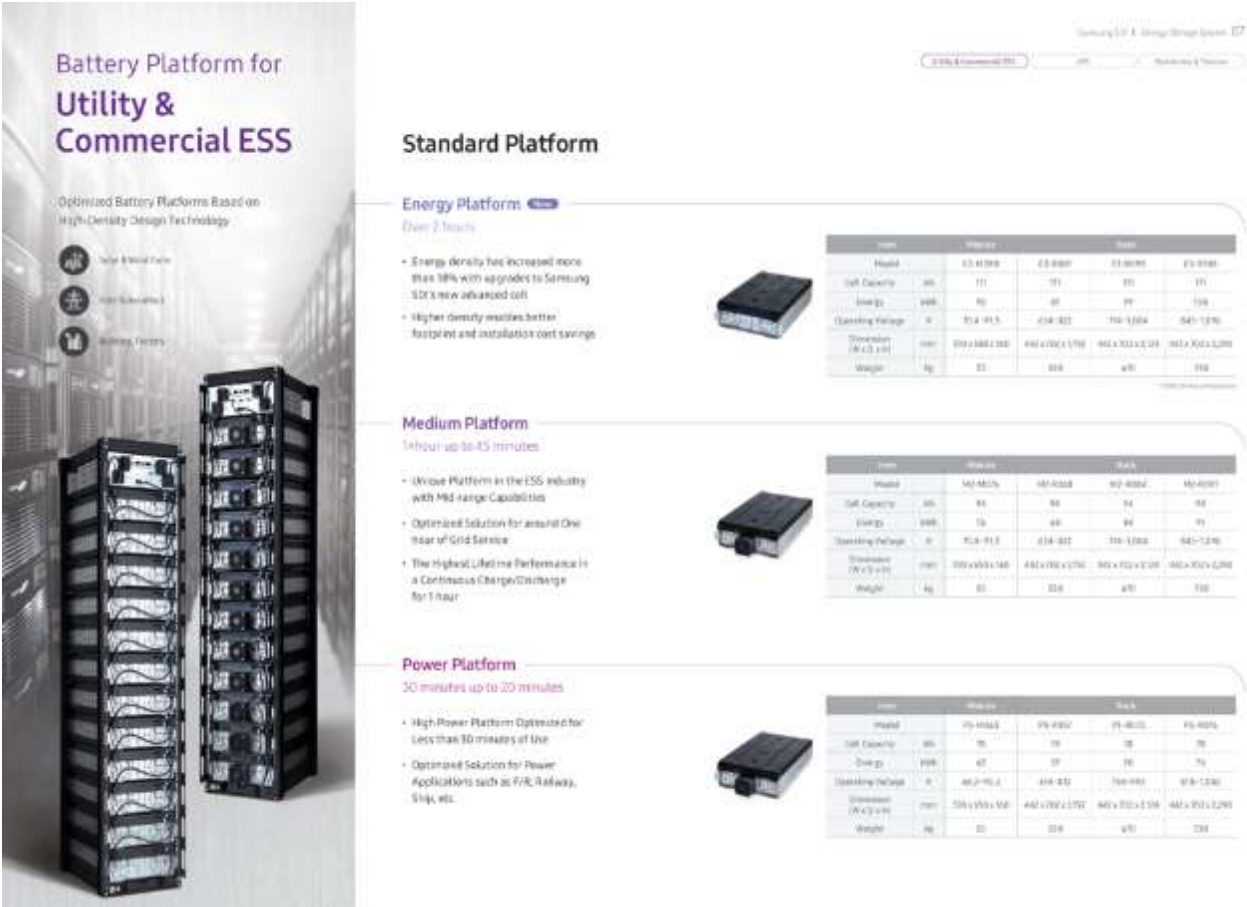
Figure A-1: Samsung Battery Specifications Sheet
