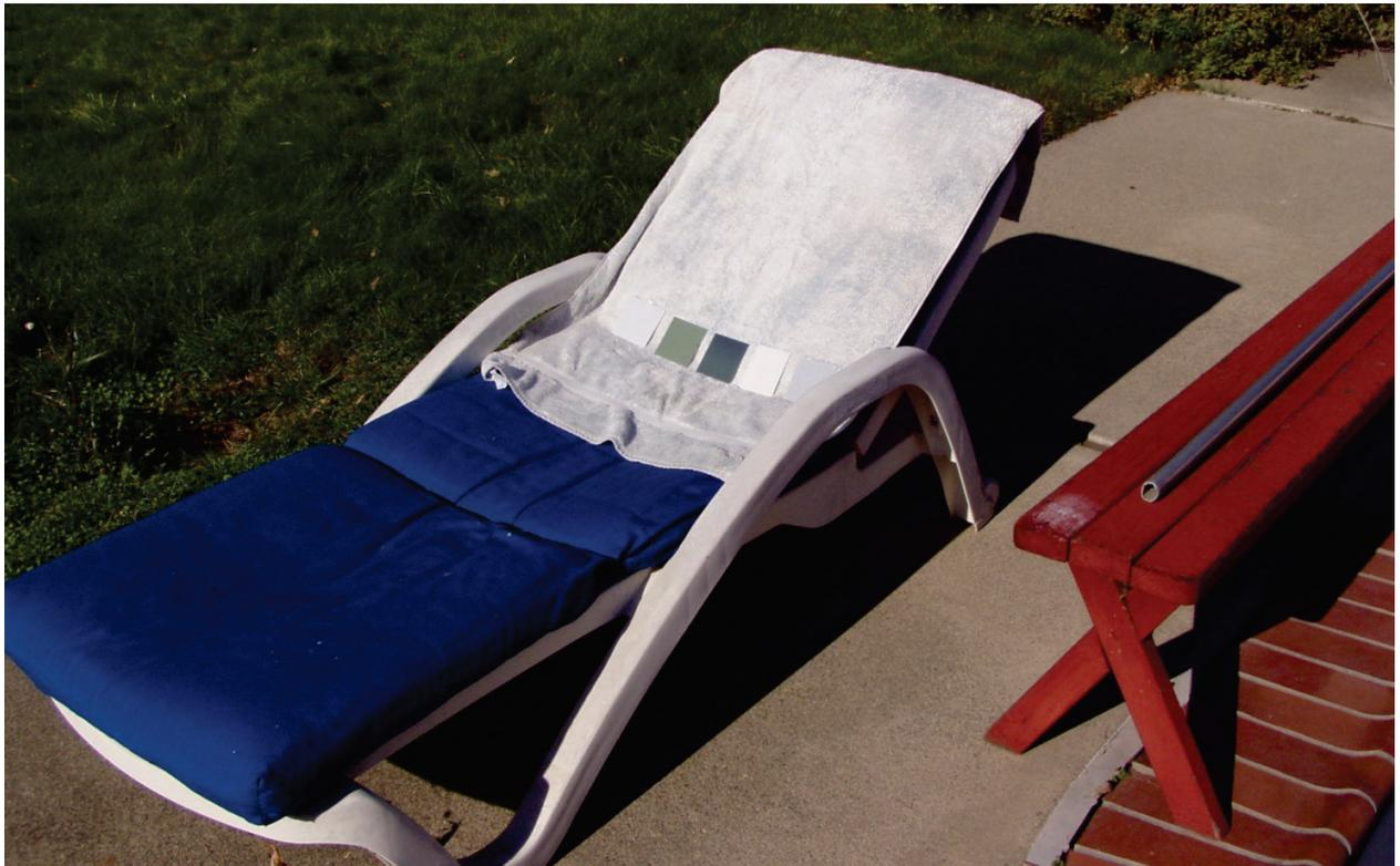
**ESM Figure A-3. Reclining chair with towel used to support specimens in Experiment 0. Note that this photo shows a set of specimens different from that used in Experiment 0.**
