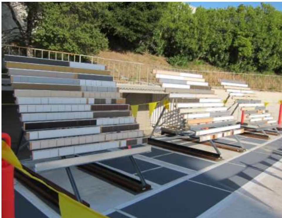
Wall-product exposure rack on building roof at Lawrence Berkeley National Laboratory.
