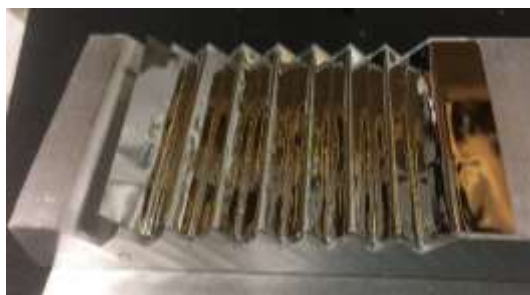
Figure 22: Example of Two-Surface Empty Mirror Retroreflector
