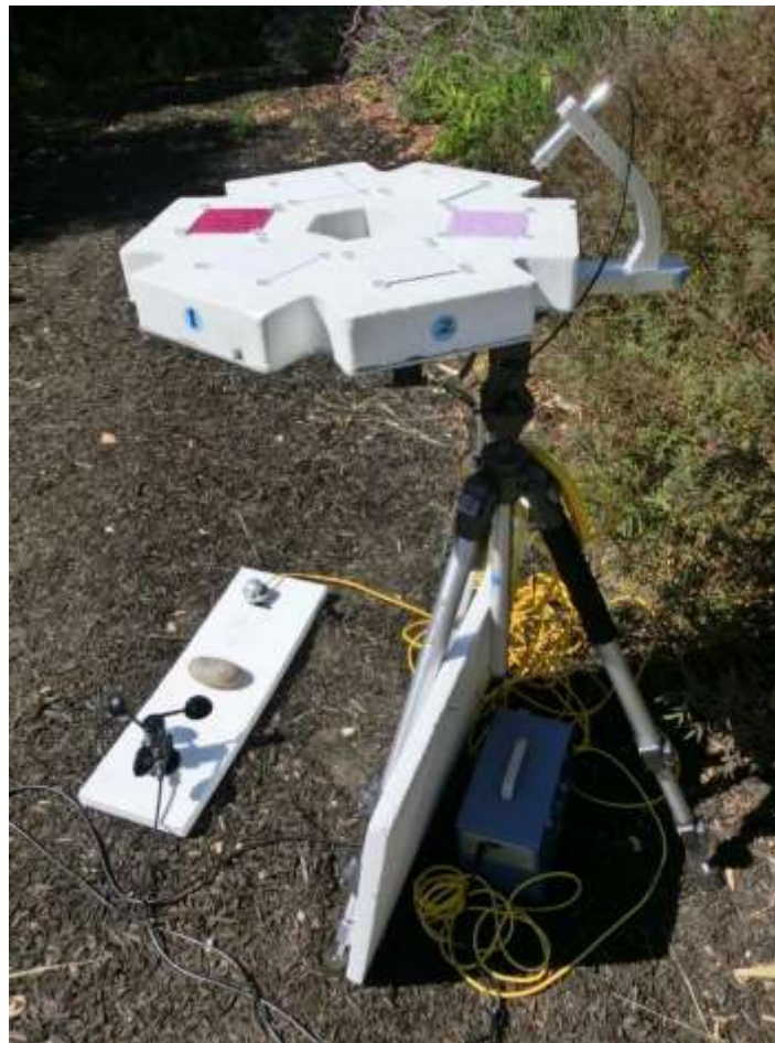
Figure 11: Apparatus for Measurement of Effective Solar Reflectance
