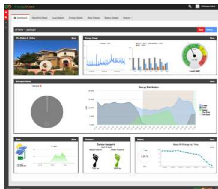
Figure 28: 13-Hour Islanding Test at Fire Station 6
