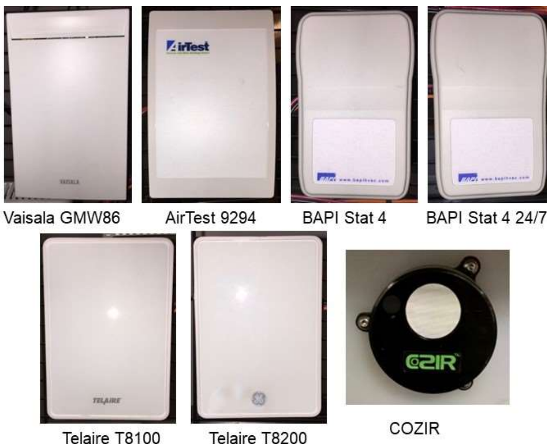
Figure 3: Selected Carbon Dioxide Sensors for Accuracy Evaluation Study
