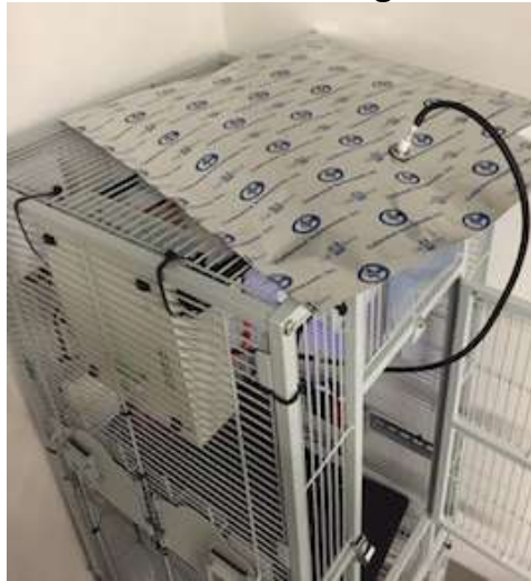
Figure 20: Carbon Dioxide Reference Instrument Accuracy Check using Calibration Bags
