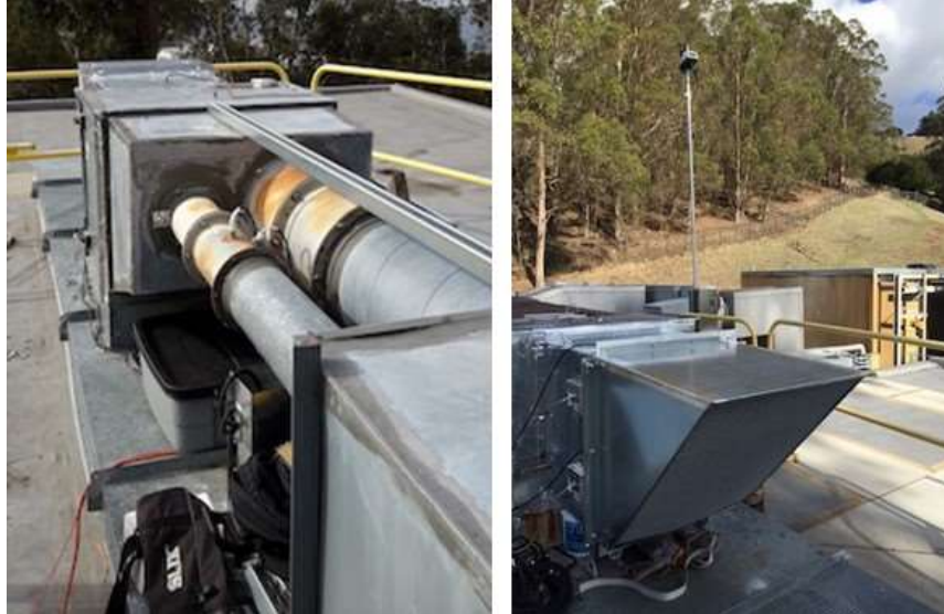
(Left) Reference flow meters consisted of a smaller 6-inch nozzle and a larger 12-inch nozzle. (Right) Onsite weather station.
