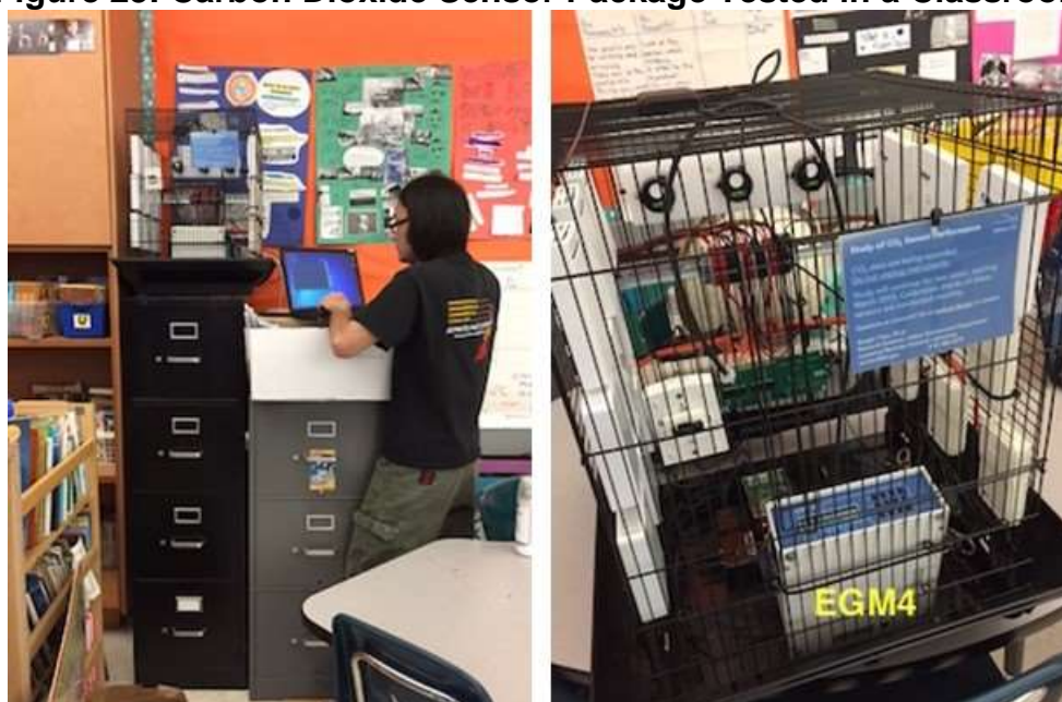
Figure 23: Carbon Dioxide Sensor Package Tested in a Classroom
