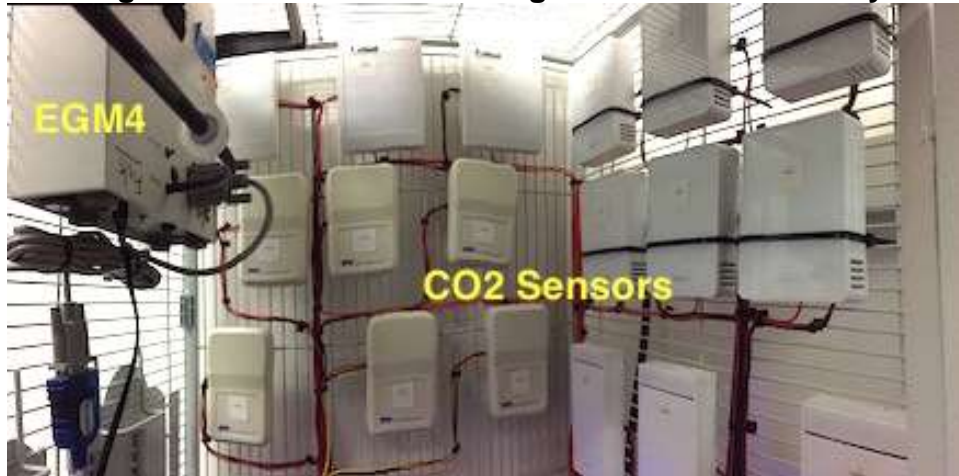
Figure 19: CO 2 Sensor Package for Evaluation Study
