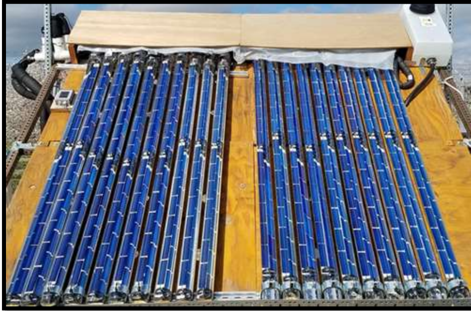
Figure 5: Micro-Combined Heat and Power Collector Testing Set-Up
