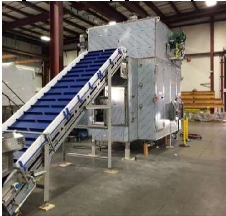
Figure 18: Hot Air Drying Section of System
