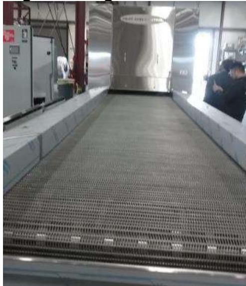
Figure 16: Front View of Infrared Heating Section of System with Conveyor for Feeding Fresh Vegetable and Fruit Slices
