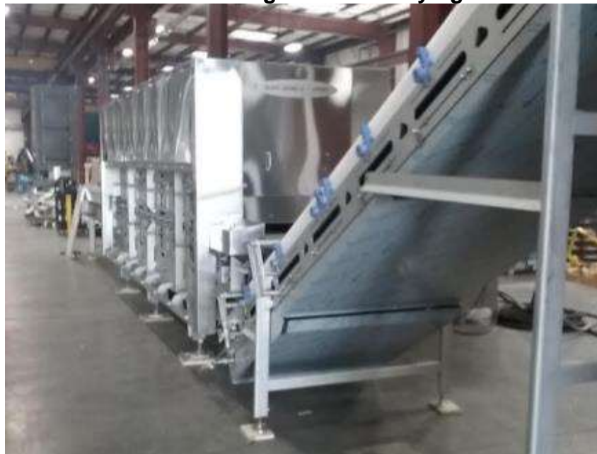
Figure 17: Rear Side of the Infrared Heating Section and the Elevator for Feeding to Hot Air Drying Section
