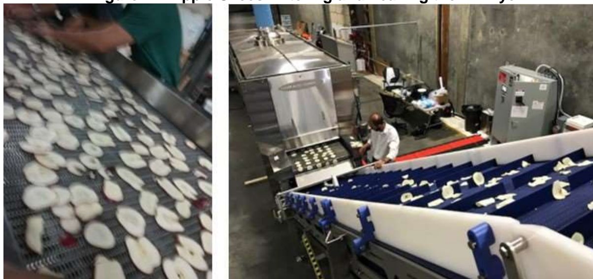
Figure 22: Apple Slices Entering and Leaving the IR Dryer
