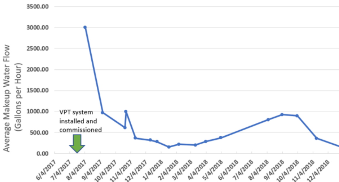
Figure 24: Makeup Measured Water Flow for the Hotel Site Marriott Average Makeup Water Flow per Hour (Measured by Carlon Totalizing Makeup Flowmeter)
