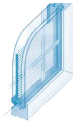
Figure 3-5: Diagram of Integrated Shading System
