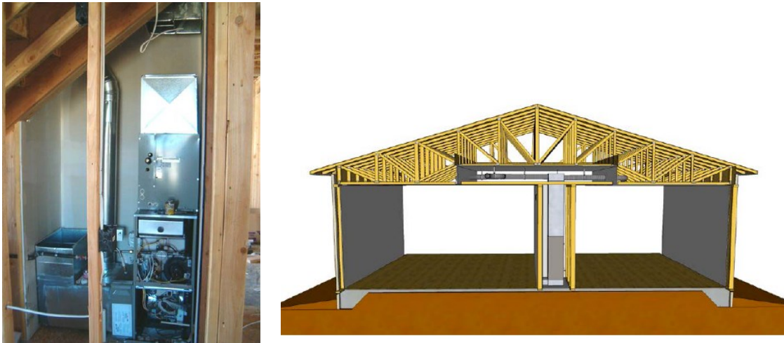
Figure 4-14: Mechanical Closet Placement Example
