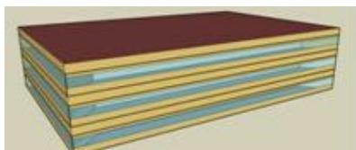
The medium office building model is a three-story rectangular building with an overall area of 53,600 square feet. It has a window-to-wall ratio of 33 percent with fenestration distributed evenly across all four façades. The zones are served by DX cooling and gas furnace heating with hot water reheat. For more details refer Appendix 3A. This prototype is used for both detailed geometry and simple geometry test cases.
