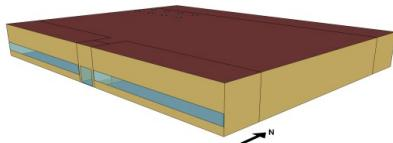
The stand-alone retail building is a single-story rectangular building measuring 178 feet by 139 feet. The total area is 24,695 square feet. Windows are located only on the street-facing façade and occupy 25.4 percent of that façade. The building is divided into five thermal zones that are served by packaged single-zone systems as described in Appendix 3A. This prototype is used for both detailed geometry and simple geometry test cases.
