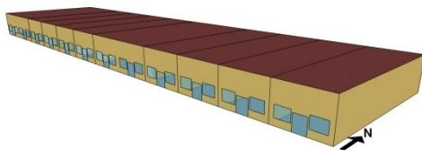
The strip mall building area is 22,500 square feet. It has 10 zones each with rooftop units. The building has windows in the street-facing façade and has an overall window-to-wall ratio of 10.5 percent. For more details refer to Appendix 3A.
