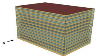
The large office building has 12 floors and a basement floor with glass windows with a window-to-wall ratio of 40 percent on the above-grade walls. The total area of the building is 498,600 square feet. The HVAC system type used is a variable air volume (VAV) system. For more details refer Appendix 3A.
