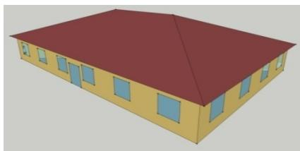
The small office building model is a single-story rectangular building of 5,500 square feet. It has punched windows and a hipped roof with an attic. There are five zones, each served by packaged single-zone air conditioner units. For more details refer Appendix 3A. This prototype is used for simple geometry test cases only.
