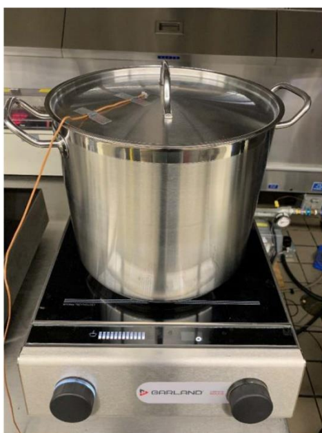
Figure D-3: Water Boil Test for Induction Cooktops
