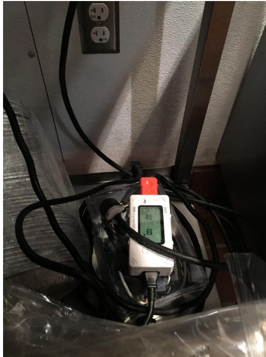
Figure 1: In-Line Plug Load Meters Installed at Chipotle
