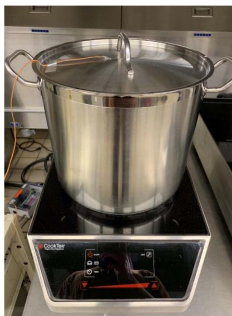
Figure D-3: Water Boil Test for Induction Cooktops
