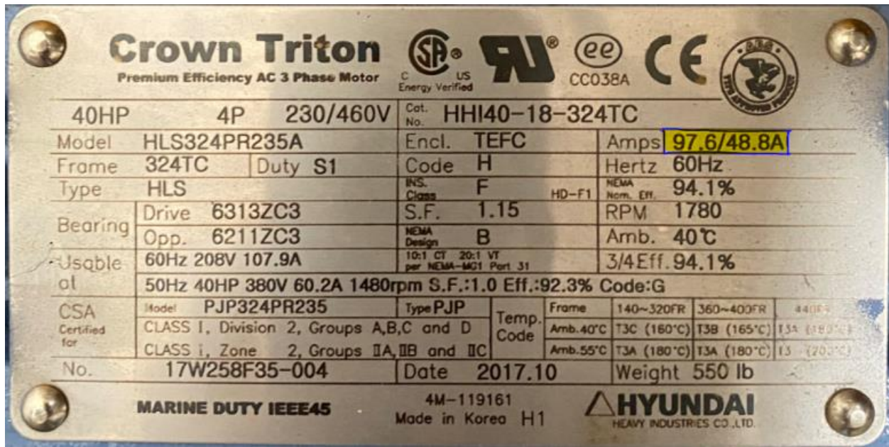
Figure 7: Induction Motor Nameplate
