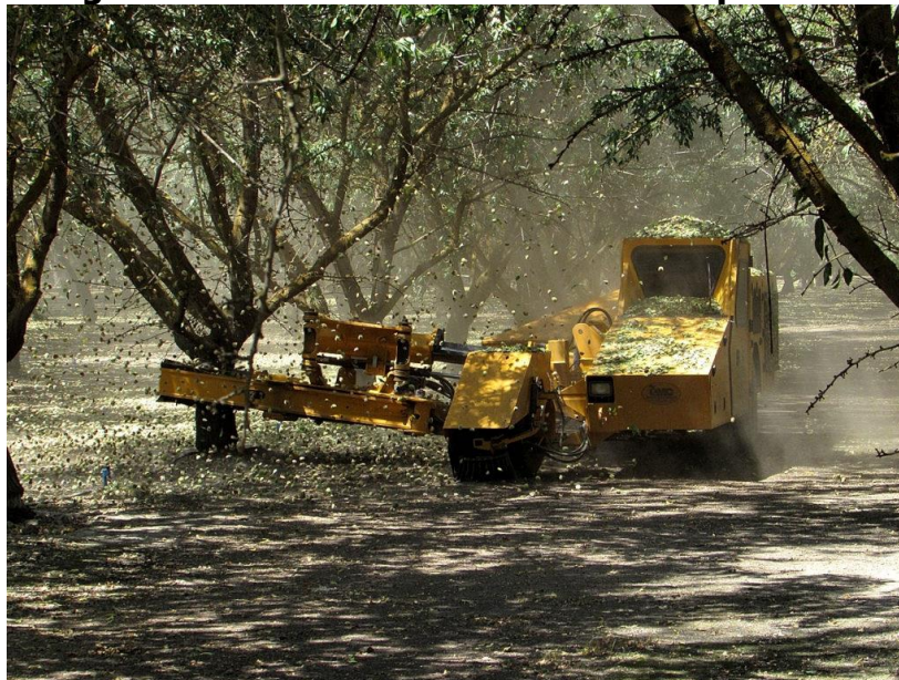
Figure 5: Diesel Powered Shaker In Operation
