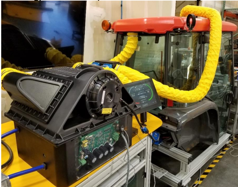
Figure 7: Heating, Ventilation, and Air Conditioning Rev 2 Test Setup
