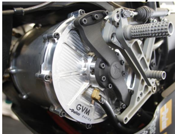
Figure 1: Global Vehicle Motor on a Victory Racing Motorcycle
