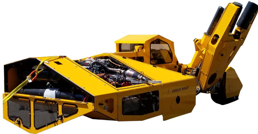
Figure 4: Compressed Natural Gas Hybrid-Electric Almond Nut Tree Shaker
