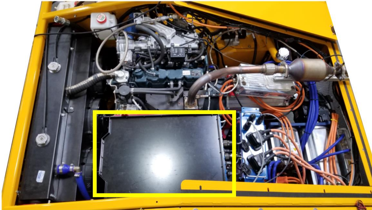
Figure 15: Ruggedized Battery Pack Location
