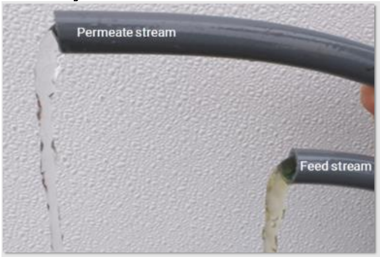
Picture of pilot permeate stream (left) and source water stream into FO module (right) Source: Porifera, Inc.
