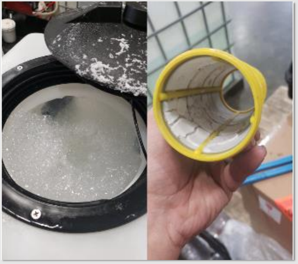
Photographs of the foamy Feed 1 (left) and the strainer (right) clogged with organics.
