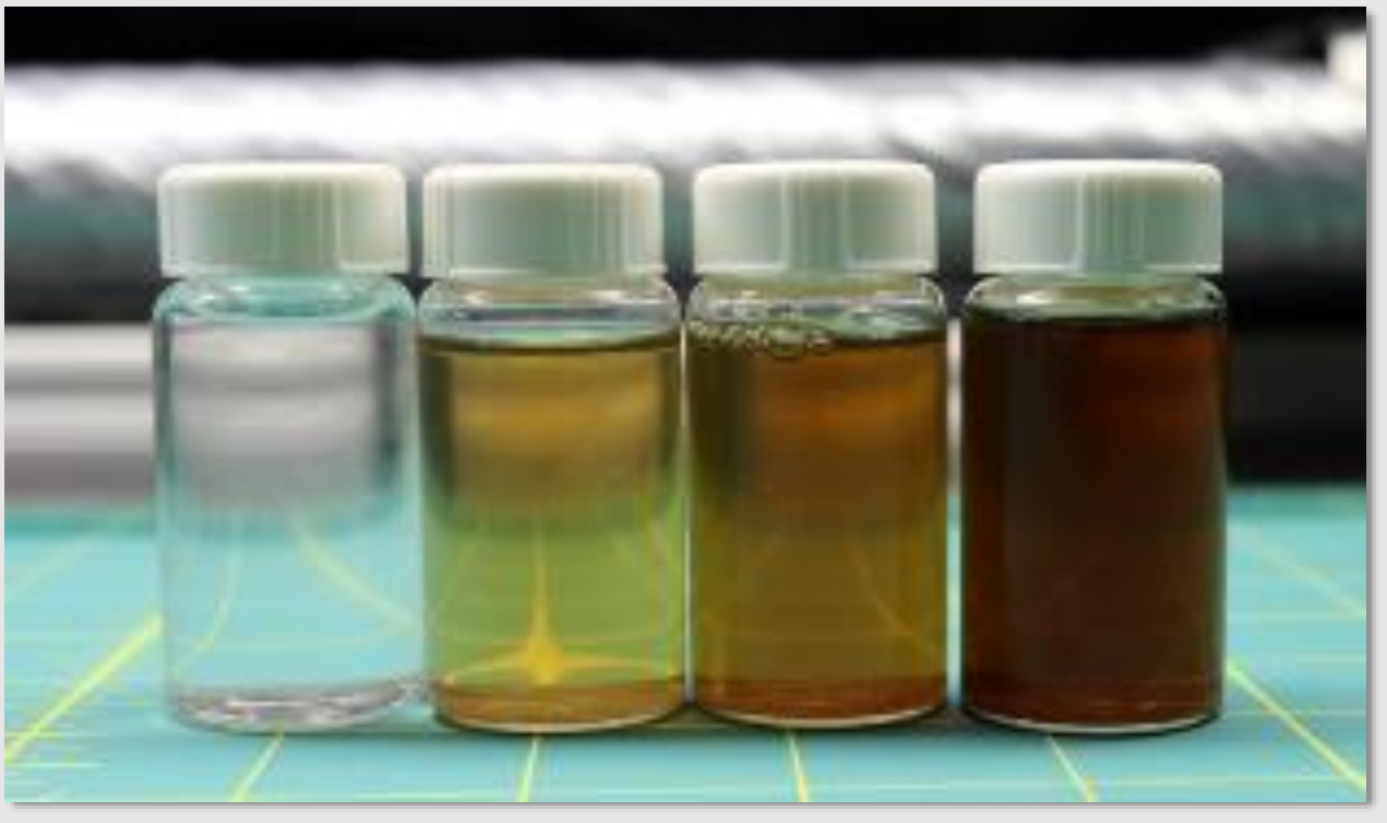
Picture of the Dilute draw (left), feed (left center), FO concentrate at 50 percent recovery (right center) & 80 percent recovery (right)
