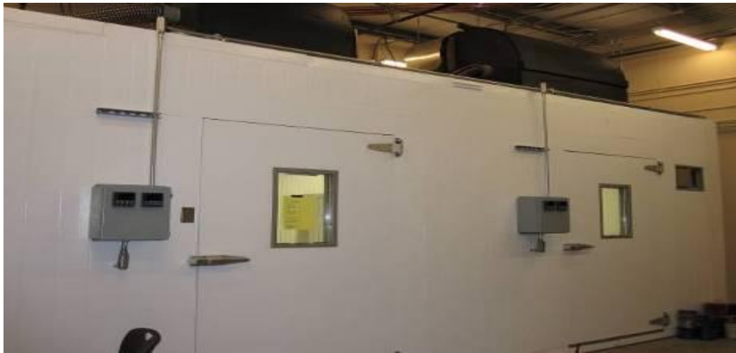
Figure 2: EPRI Thermal Chambers Used in Experimental Setup
