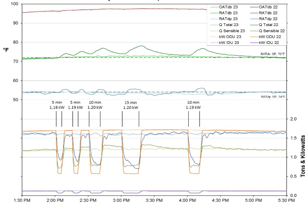
Figure B-8: Detail of Dynamic Cooling Test #13 (with Realistic Temperature Profile)
