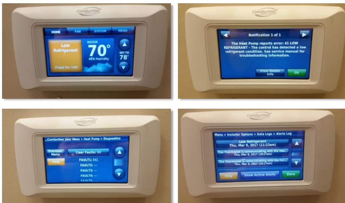
Figure 90: Thermostat Displays of Low Refrigerant Fault in Heating Mode
