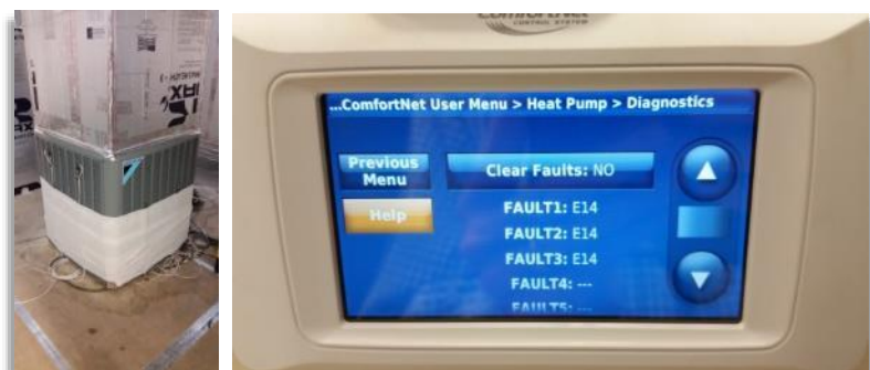
Figure 83: Applied Outdoor Airflow Restriction and Thermostat Diagnostic Page
