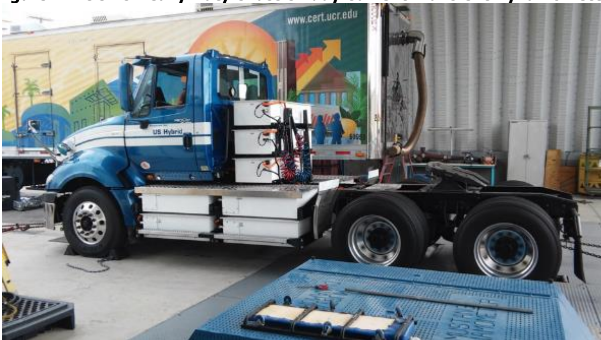
Figure 74: UCR's Heavy Duty Chassis Eddy Current Transient Dynamometer
