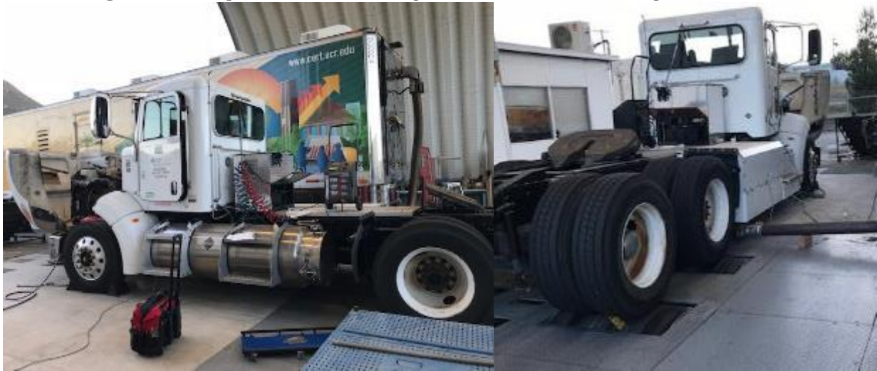
Figure 76: Hybrid Truck Setup on UCR's Chassis Dynamometer
