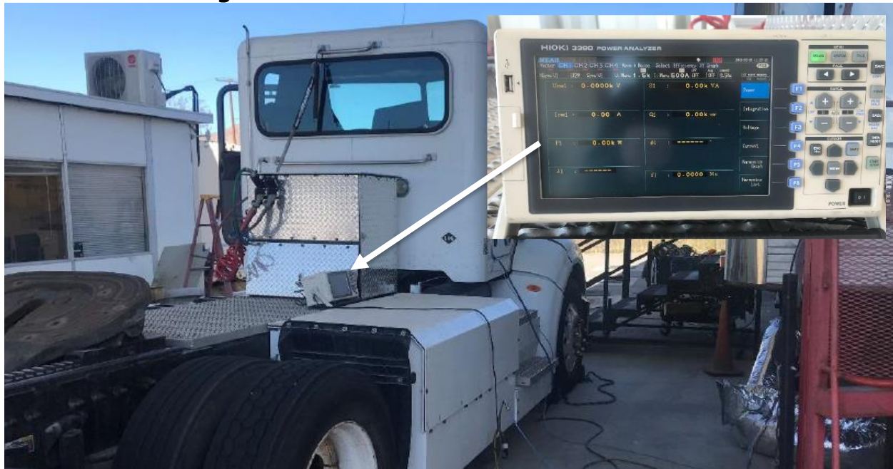
Figure 82: Installation of Hioki Power Meter
