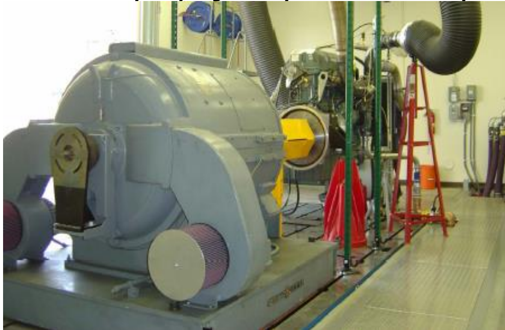
Figure 53: UCR's Heavy Duty Engine Eddy Current Transient Dynamometer
