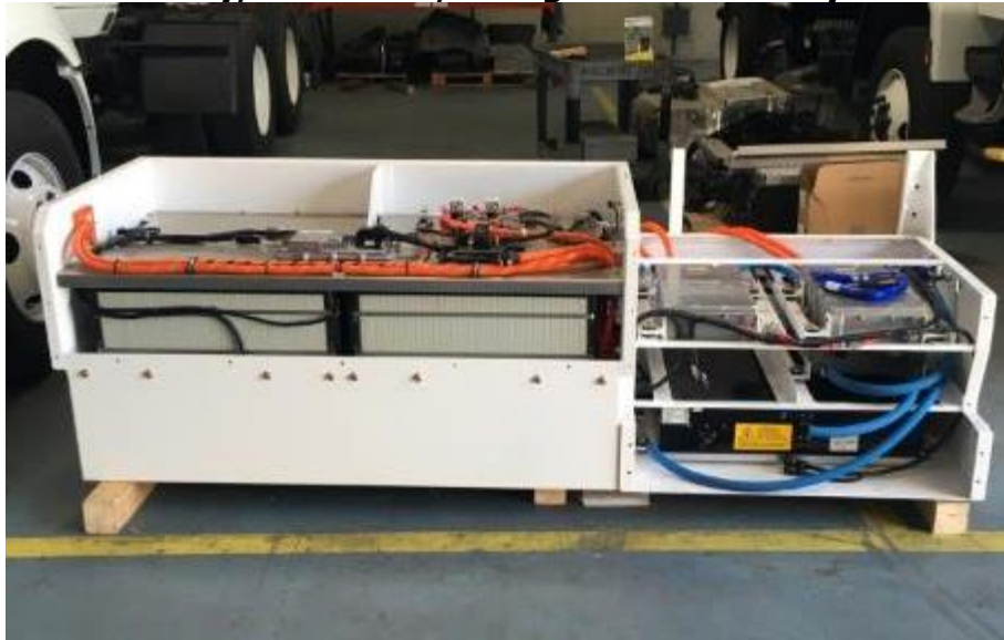
Figure 42: Battery, Controller, Charger and Auxiliary Drive Housing
