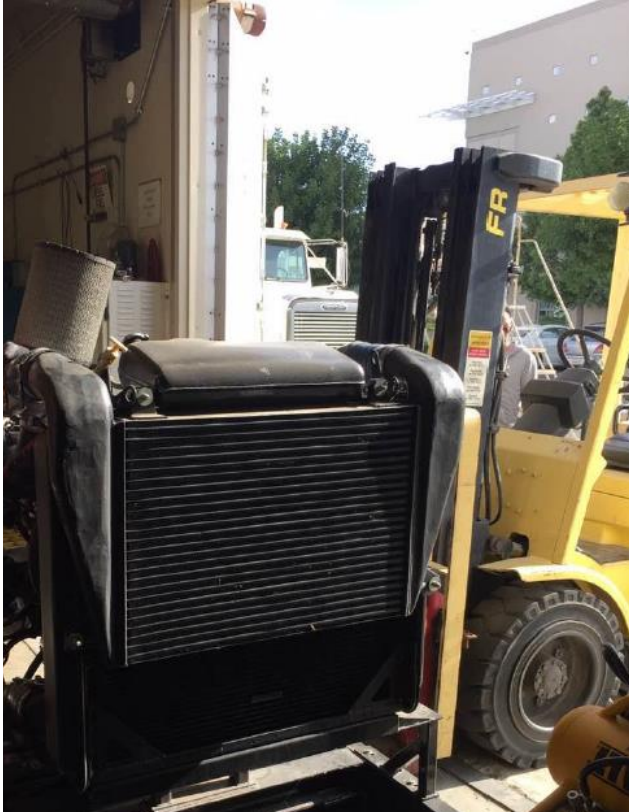
Figure 54: Fork Lifting Engine into Test Cell and Installing Customized Mounts
