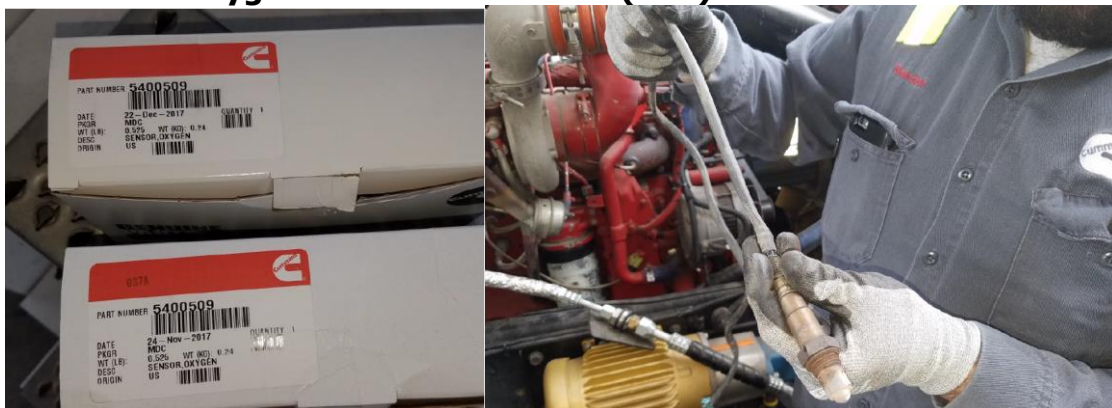
Figure 77: New Oxygen Sensors in the Box (Left) and Prior to Installation (right)
