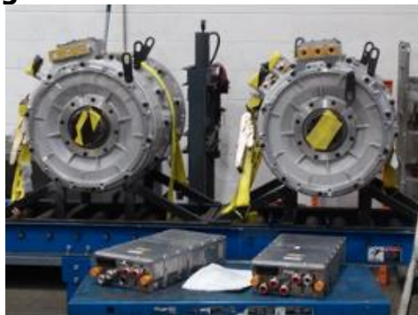
Figure 37: Motors and Controllers
