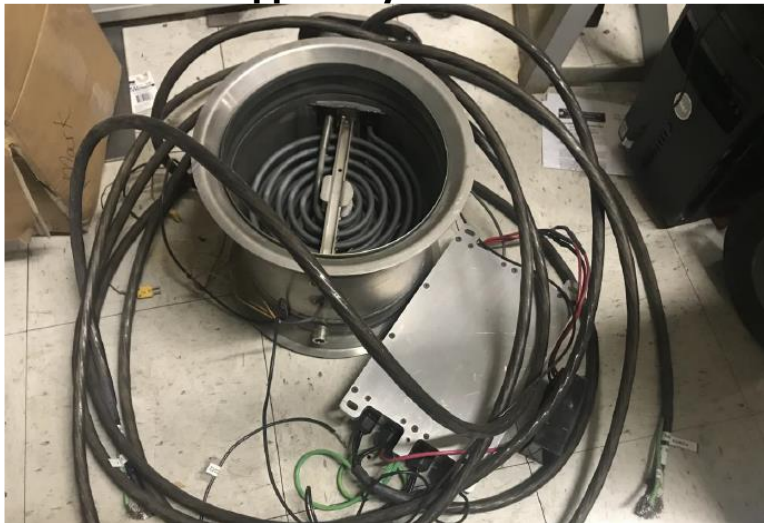
Figure 70: Heater Section Supplied by Watlow for Cold Start Improvement
