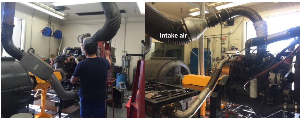
Figure 55: Engine Setup with Connections to Laboratory Services and Aftertreatment
