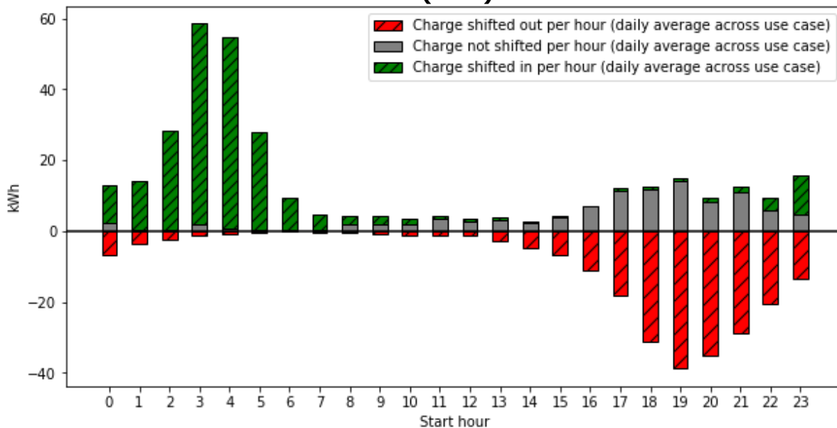
Figure 21: Vehicle Charging Energy Shifted by Hour per Day in Home 24-Hour Use Case (kWh)
