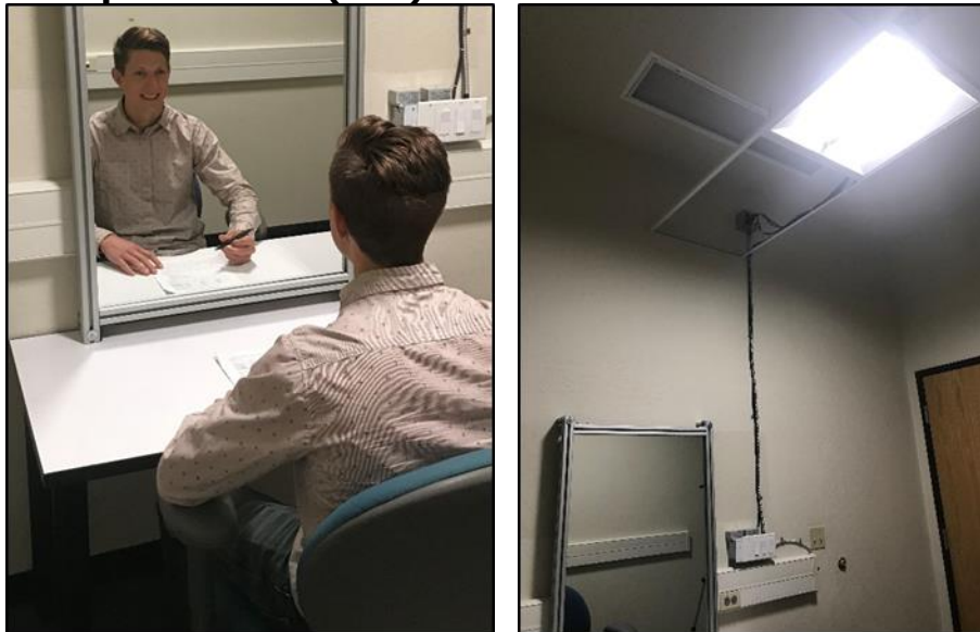
Figure 72 shows a CLTC researcher participating in the skin inspection test (left) and the ambient luminaire in the space above the mirror (right).
