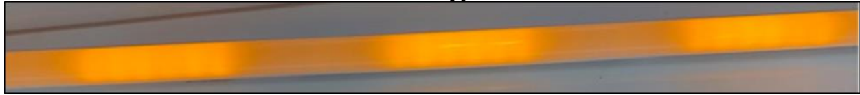
Figure 70: Uneven Lighting Distribution at Low Dim Level in the Amber Linear LED Prototype
