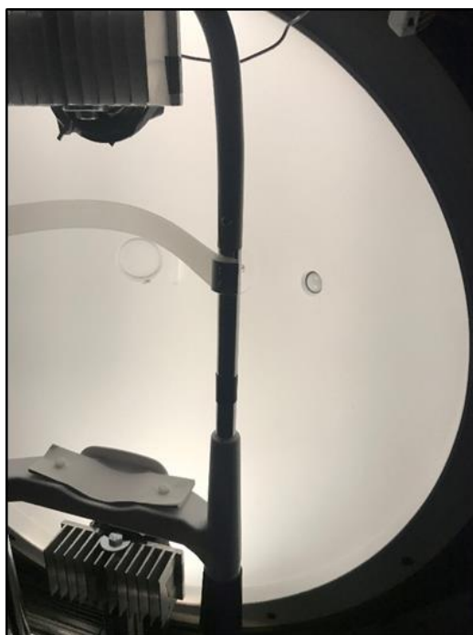
Figure 51: View of the Inside of the Sphere and the Chinrest Used for Visible-Flicker Study
