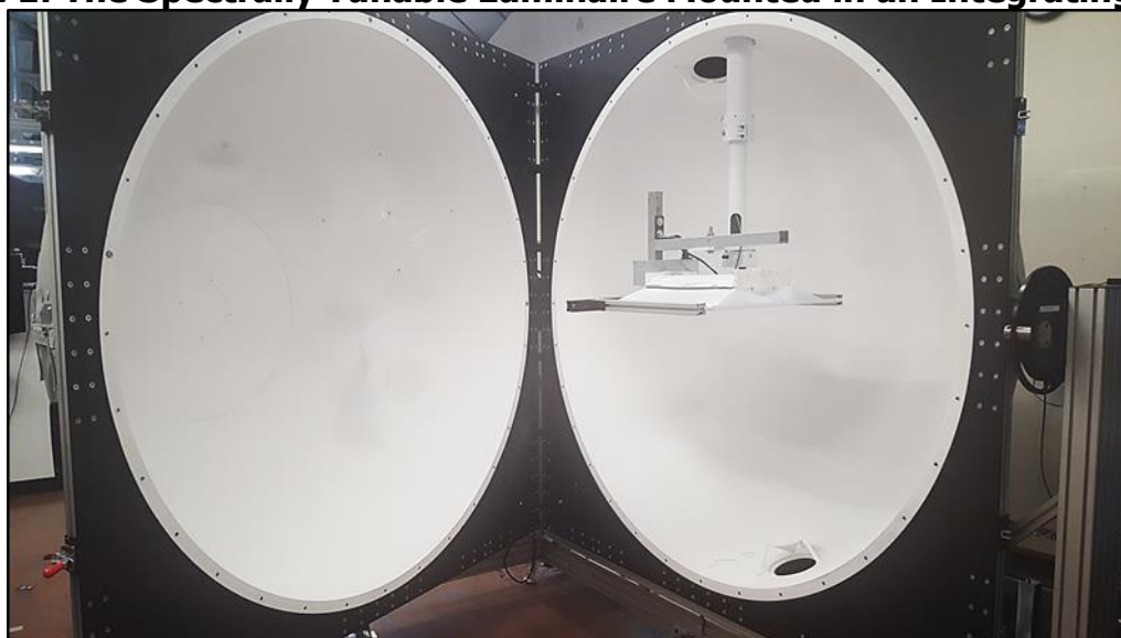
Figure 71 shows the spectrally tunable luminaire mounted in the integrating sphere for photometric and electrical characterization.
