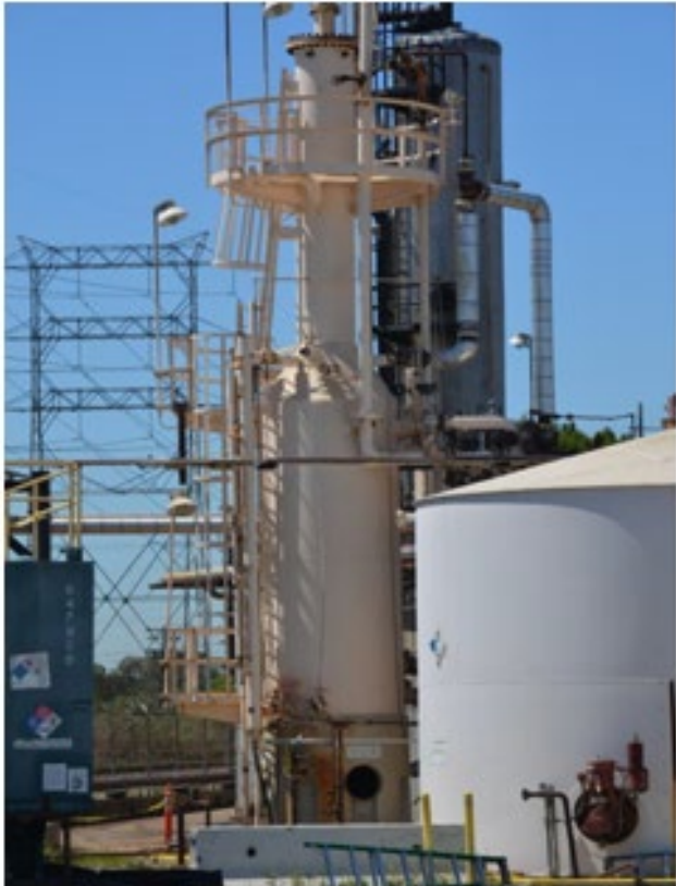
Figure 13: Reworked Support Units Including Caustic Scrubber, Sidecut Stripper, Caustic burner, and SOX Burner Unit.
