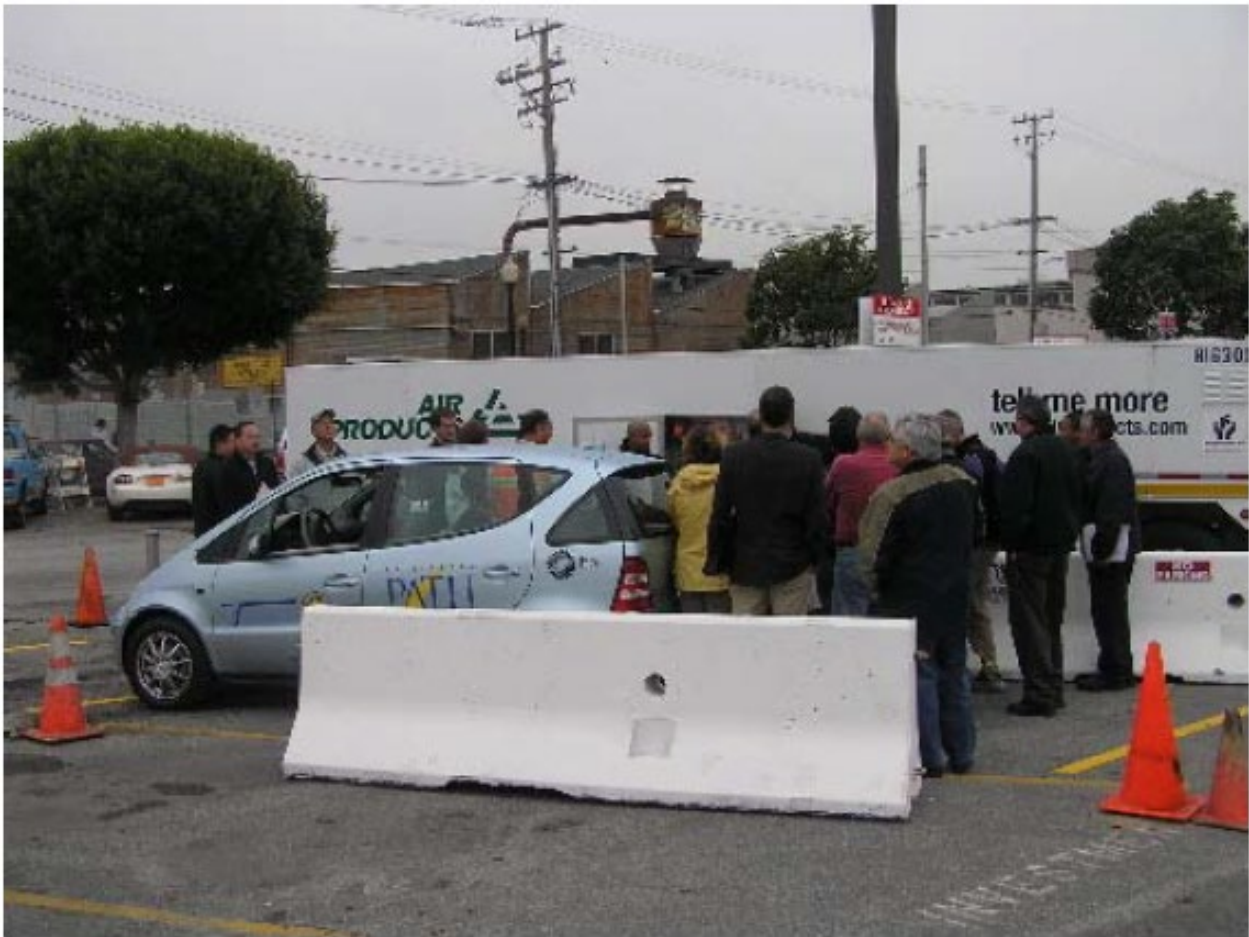
Figure 14: Mobile Hydrogen Refueler (350 Bar) at PG&E in 2006
