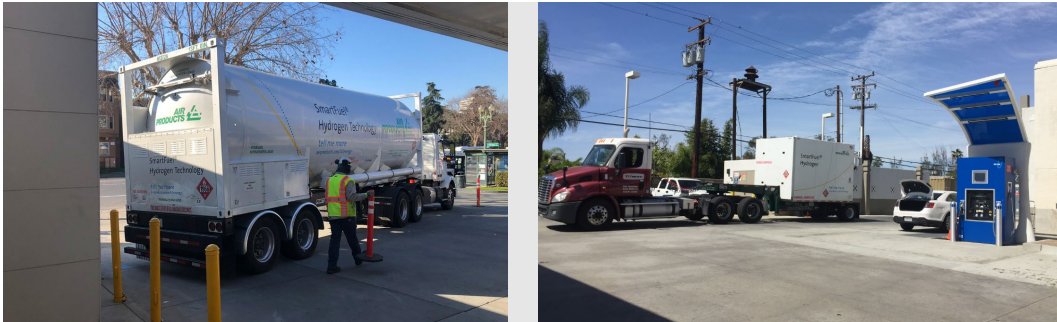
Figure 1: Liquid Hydrogen and Gaseous Hydrogen Delivery Trucks
