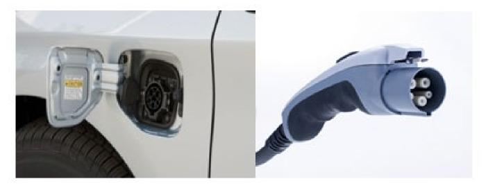
Figure 20: Level 2 Charging Connector and Inlet
