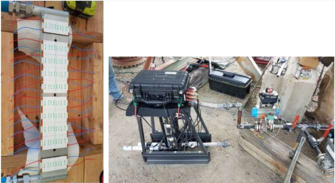
Figure 7: 240 W Geothermal-TEG Apparatus Deployed at Bottle Rock Geothermal Field, July 2019.
