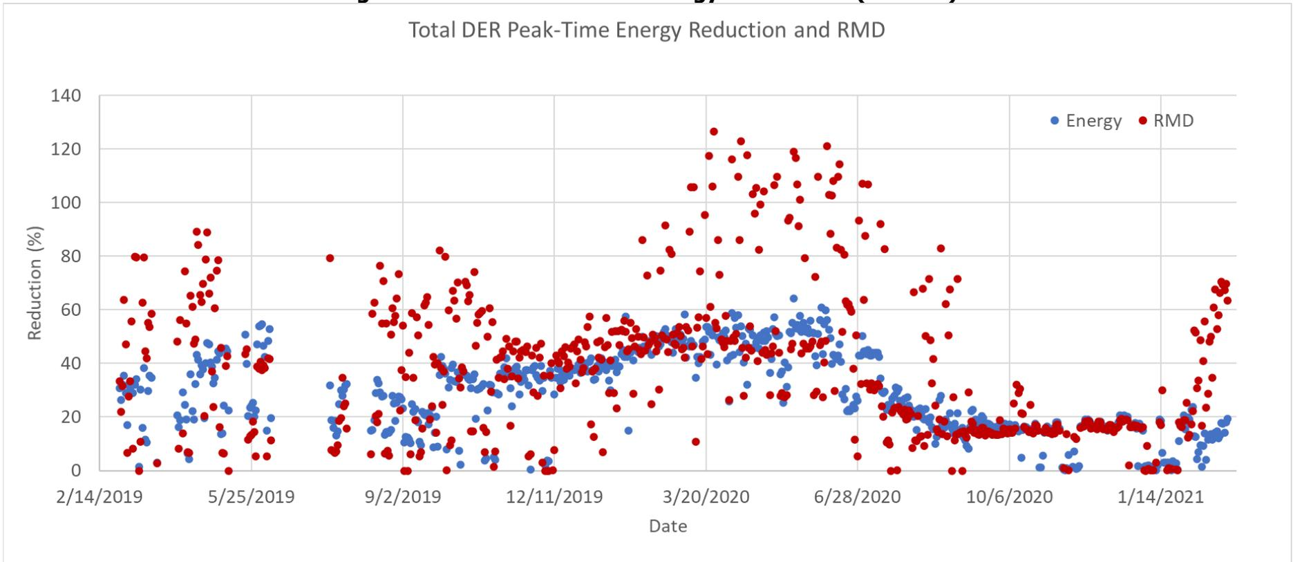
Scatter chart of reductions in peak-time energy use and RMD from solar PV paired with battery.
