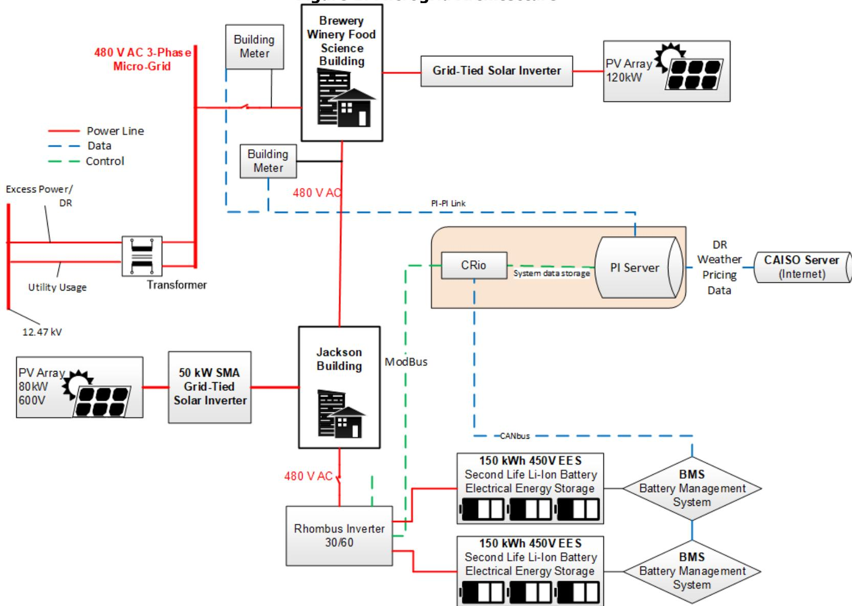
Microgrid system architecture showing power, data, and control connections.
