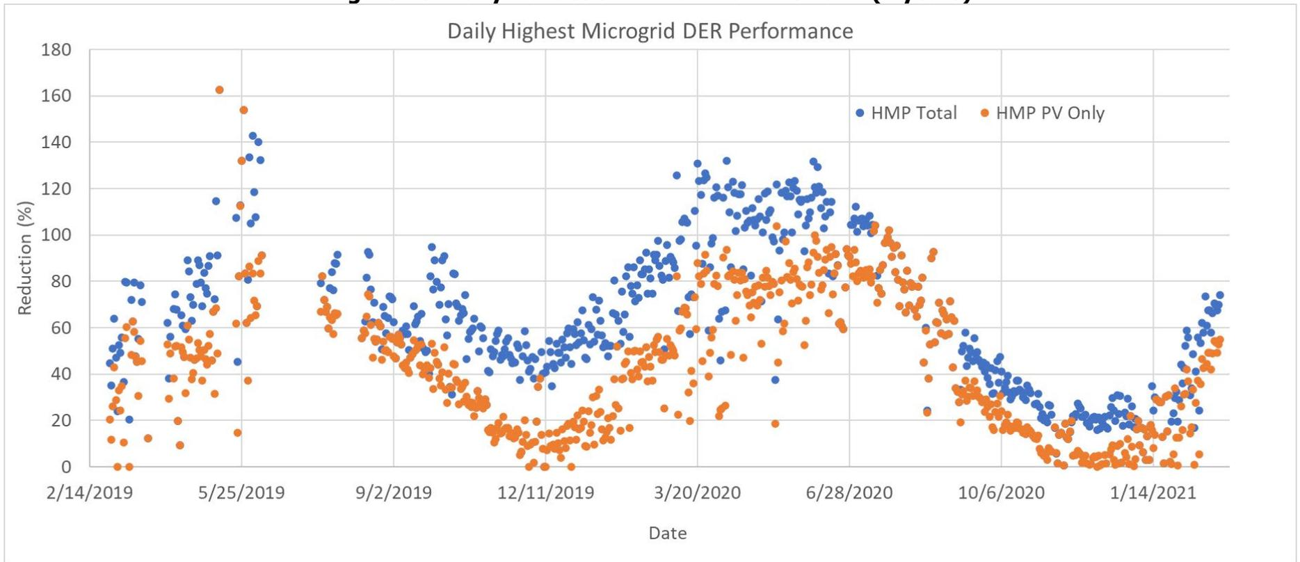
**Highest Microgrid Performance (HMP) during peak hours showing the difference between PV only and PV+ESS installed in the microgrid.**
