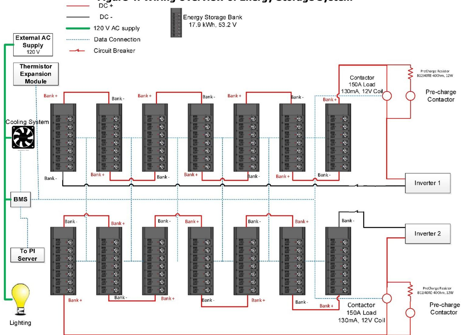
Diagram of ESS System showing banks connected in series along with BMS gathering data from the banks and sending data to PI server.
