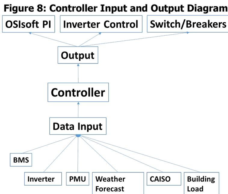
**Controller input/output Communications with other devices and databases.**
