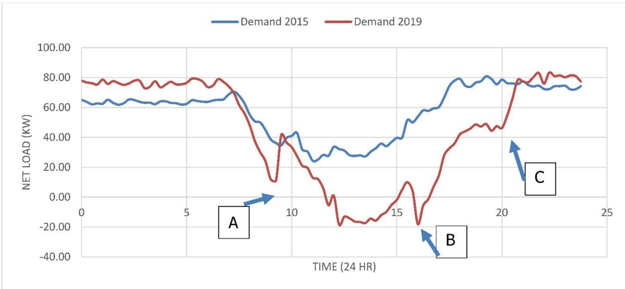
**Microgrid load data before and after system installation. Data for October 6, 2015 and October 6, 2019.**
