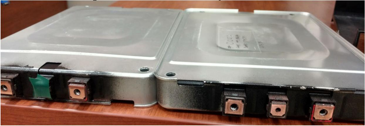
Nissan LEAF battery modules. Left: bottom of module. Right: Top of module.
