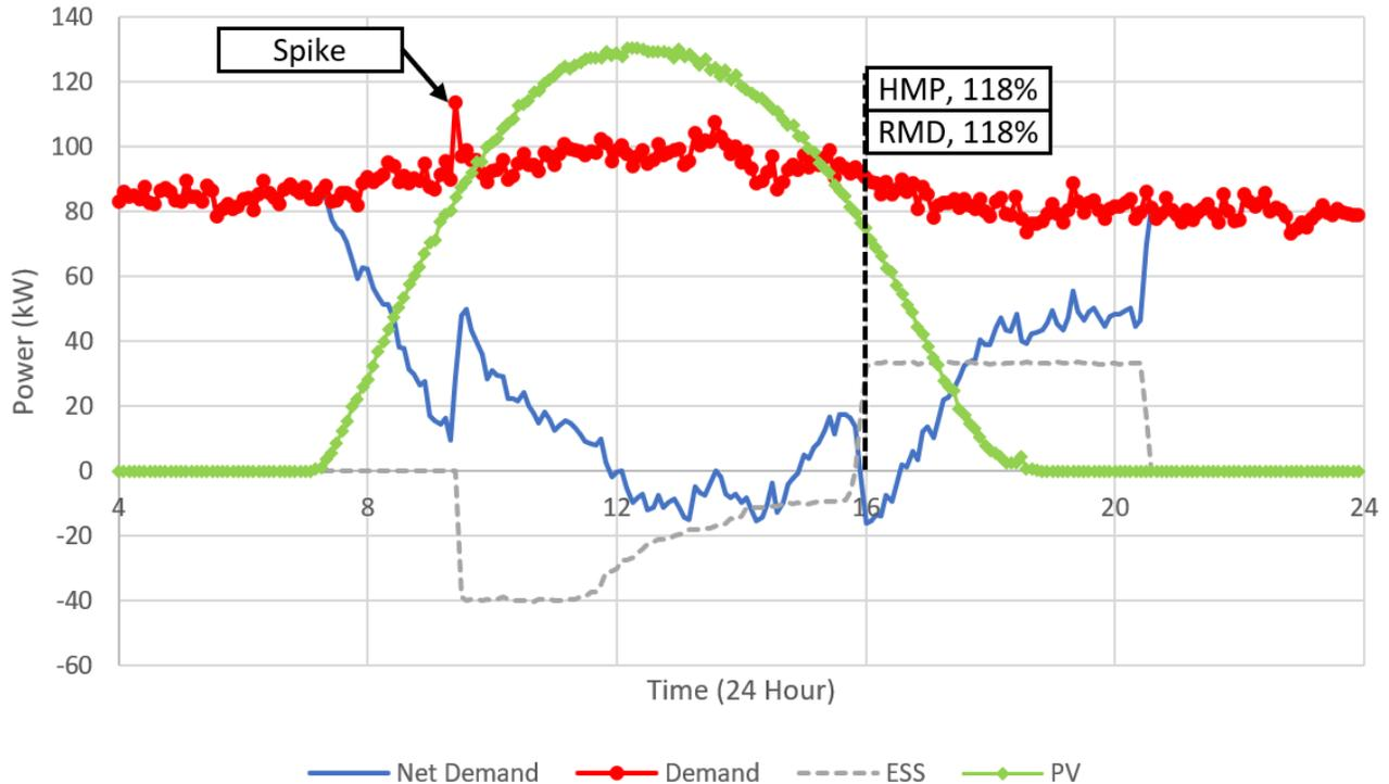
5-minute resolution power data from the microgrid October 5, 2019 showing operation during a sunny day. Negative battery power indicates charging. While it appears as if the HMP and RMD?? is caused by the data misalignment spikes mentioned, this point was not immediately when the battery turned on. The point labeled “Spike” was caused by the battery shutting off, not an actual increase in demand, this would create a false measurement of RMD.
