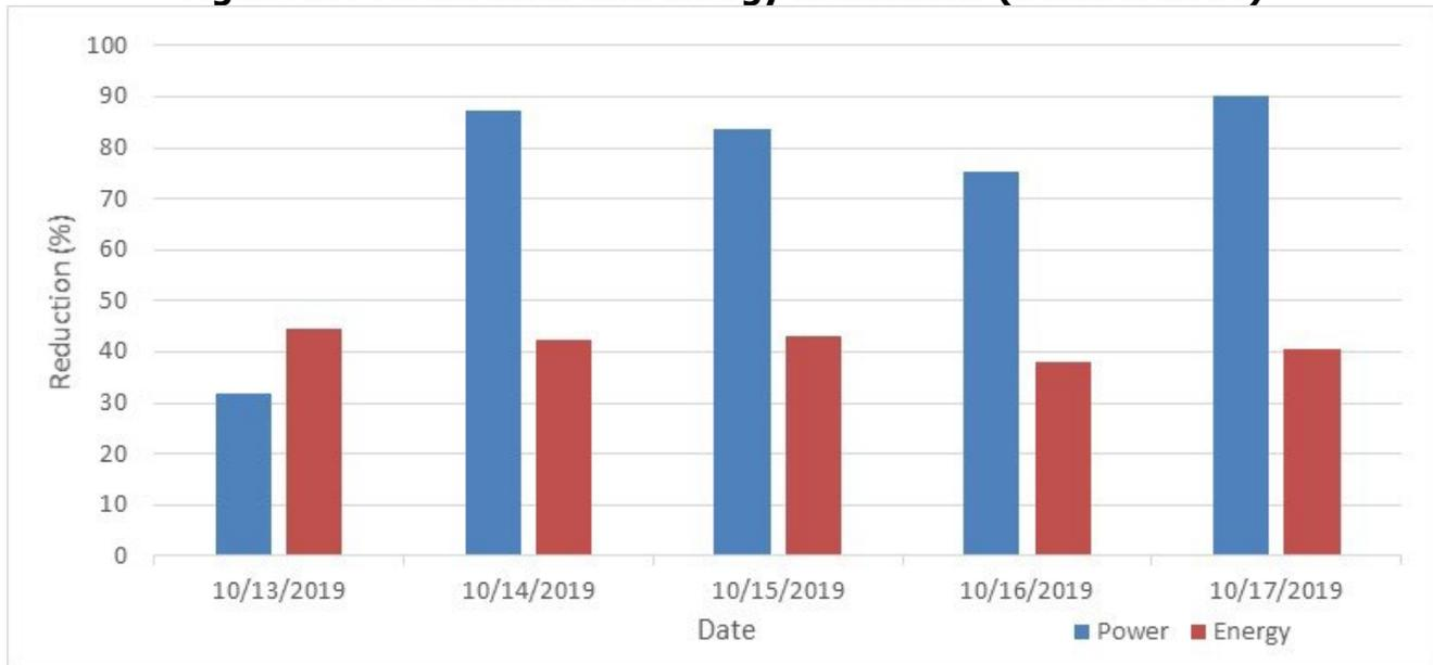
Plot of reductions in peak-time energy use and RMD from solar PV paired with battery. Plot shows zoomed in values from Figure 14 during the October 2019. “Power” refers to RMD, “Energy” refers to peak-time energy usage reduction.
