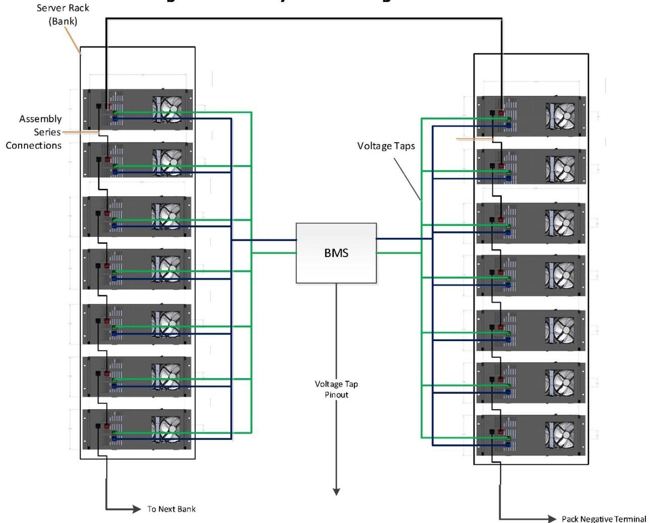
**Detailed diagram of ESS connection to BMS voltage taps and assembly series connections.**
