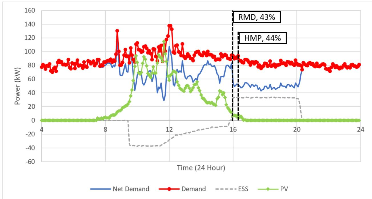
**5-minute resolution power data from the microgrid showing operation during a cloudy day. Negative battery power indicates charging.**
