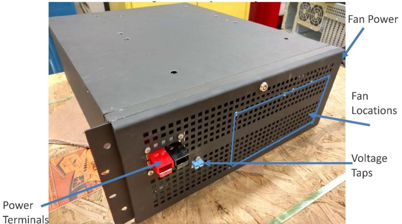
An assembly of Nissan LEAF Modules. It contains 8 modules connected in parallel. The large connectors on the front are the assembly terminals, the small blue ports are the voltage taps for the BMS.
