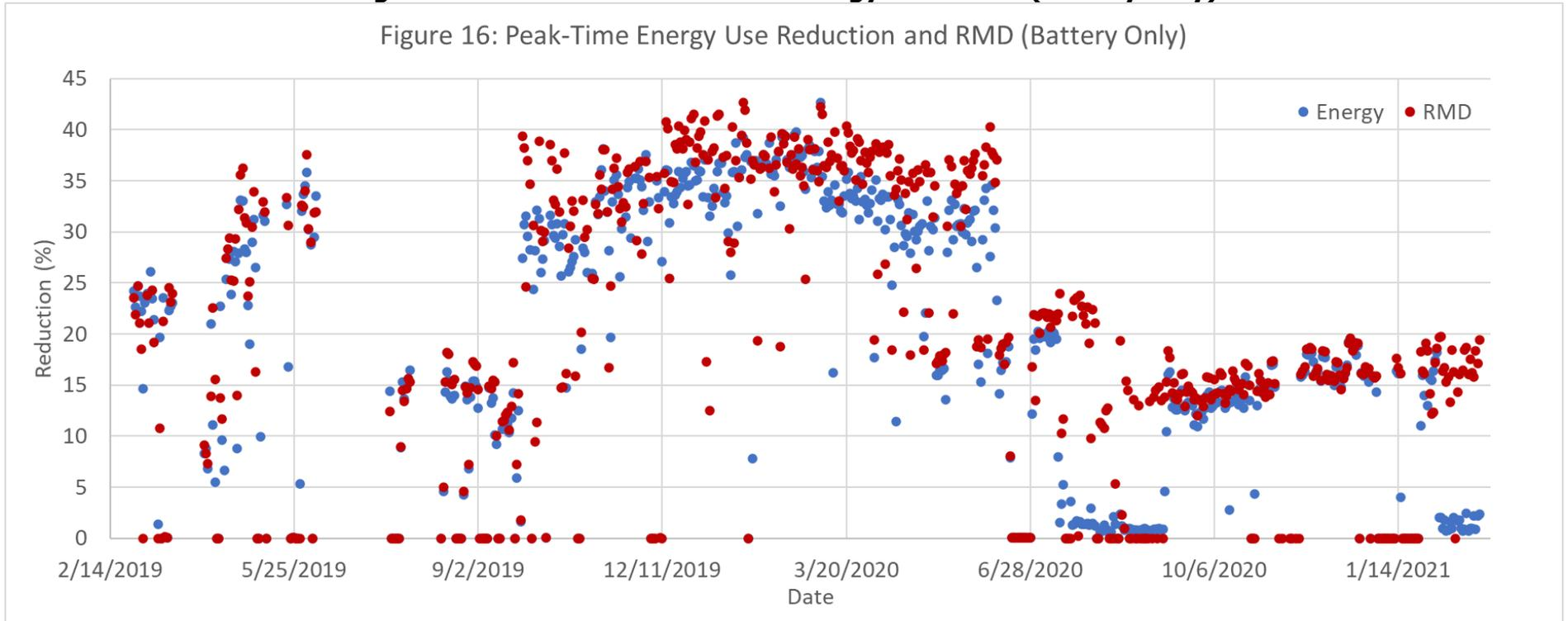
Reduction in maximum demand (RMD) and total peak time energy reduction provided by battery installation over 2 years.
