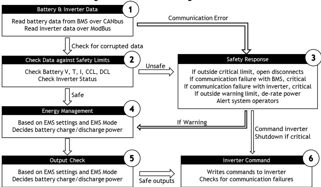
**Controller architecture diagram highlighting safety features.**
