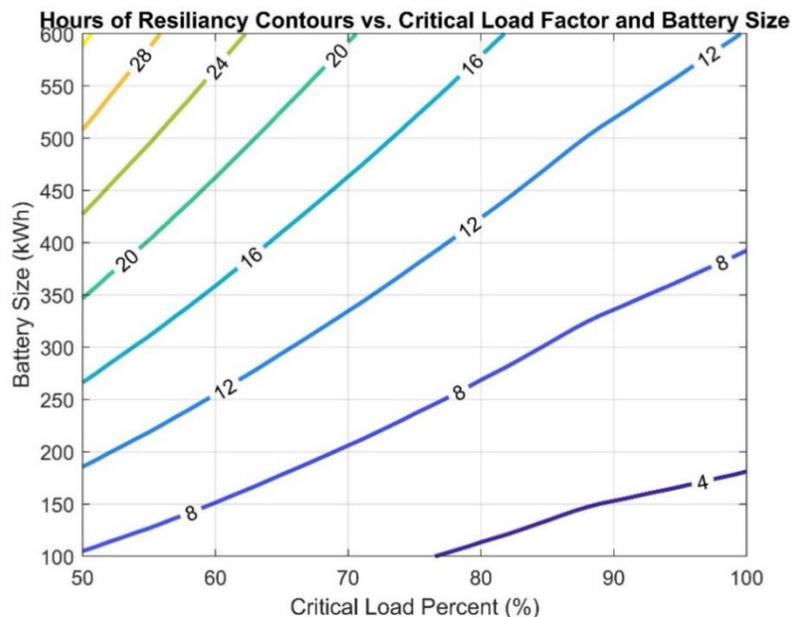
Contour plot showing how critical load factor and battery size affect backup power capability of the site. Numbers on the contour lines represent the number of hours the microgrid could run without a grid connection.
