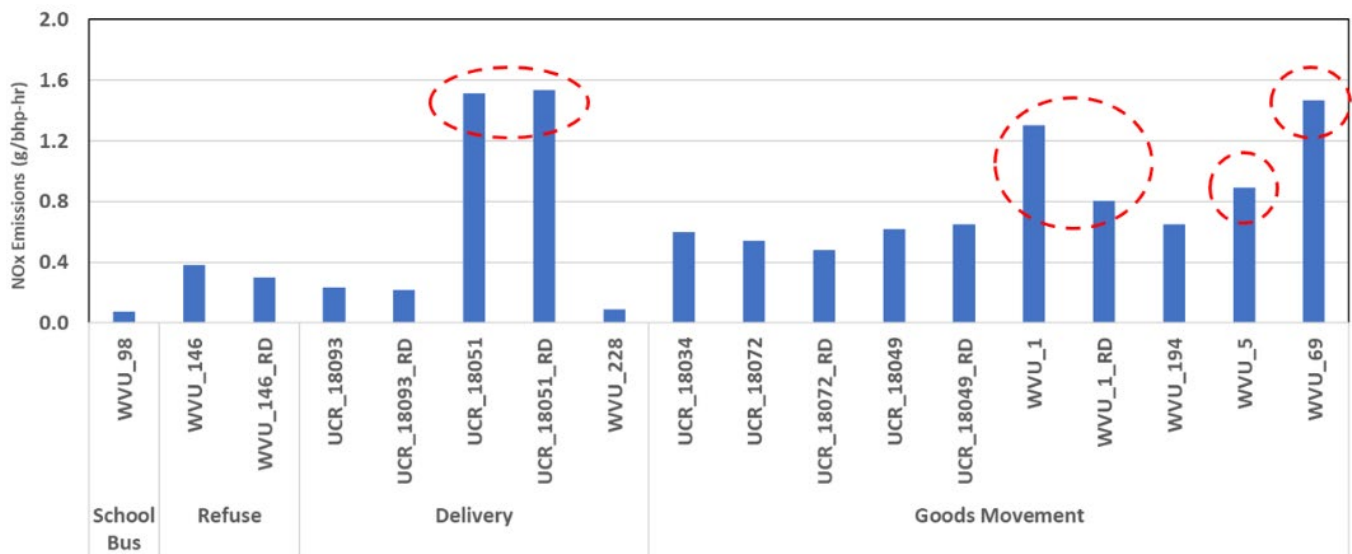
Figure 40: Cycle Averaged NOx Emissions for 0.2g Diesel HDVs (UDDS)
