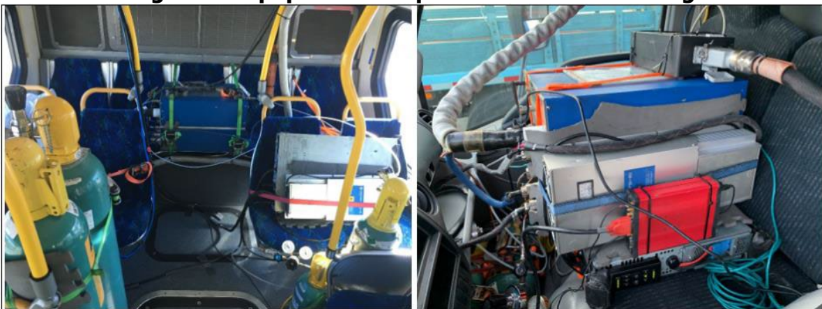
Figure 8: Equipment Setup of WVU's PEMS Testing
