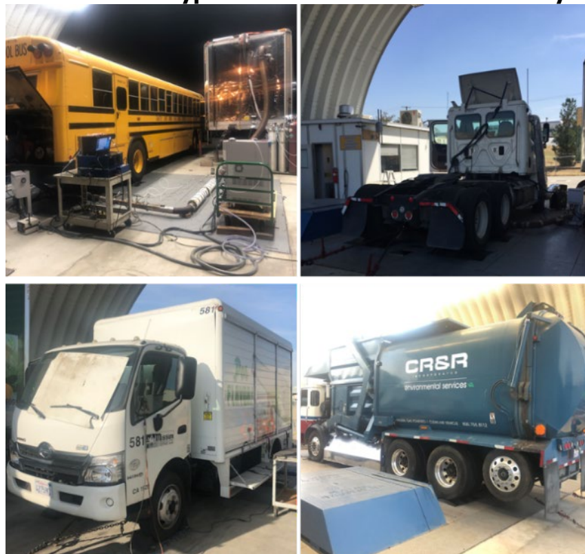
Figure 10: Various HDV Types Installed on UCR's Chassis Dynamometer
