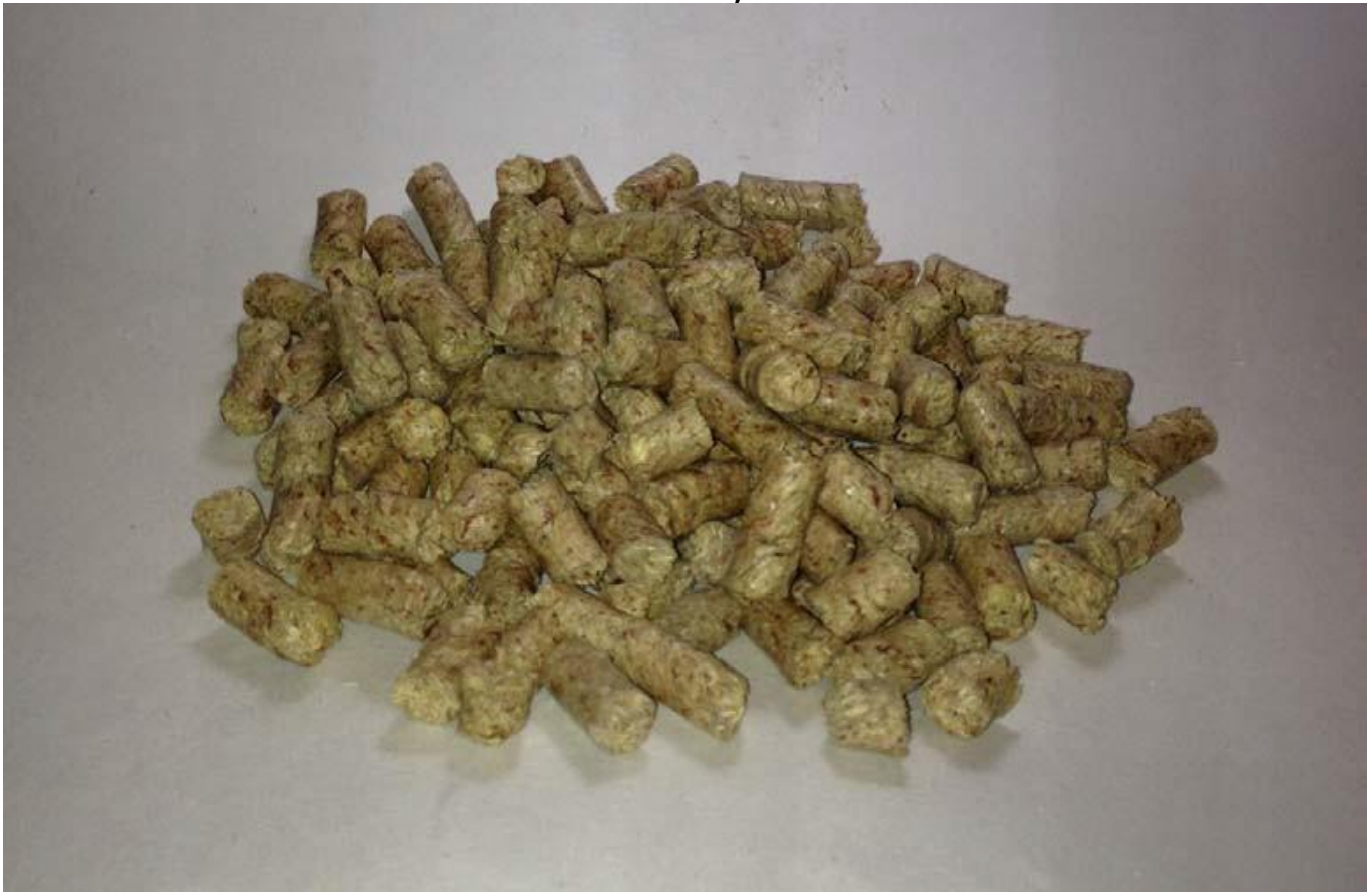
Figure 12: Densified Biomass from Sweet Sorghum Stalk Processed at Pilot Plant, Bakersfield, CA
