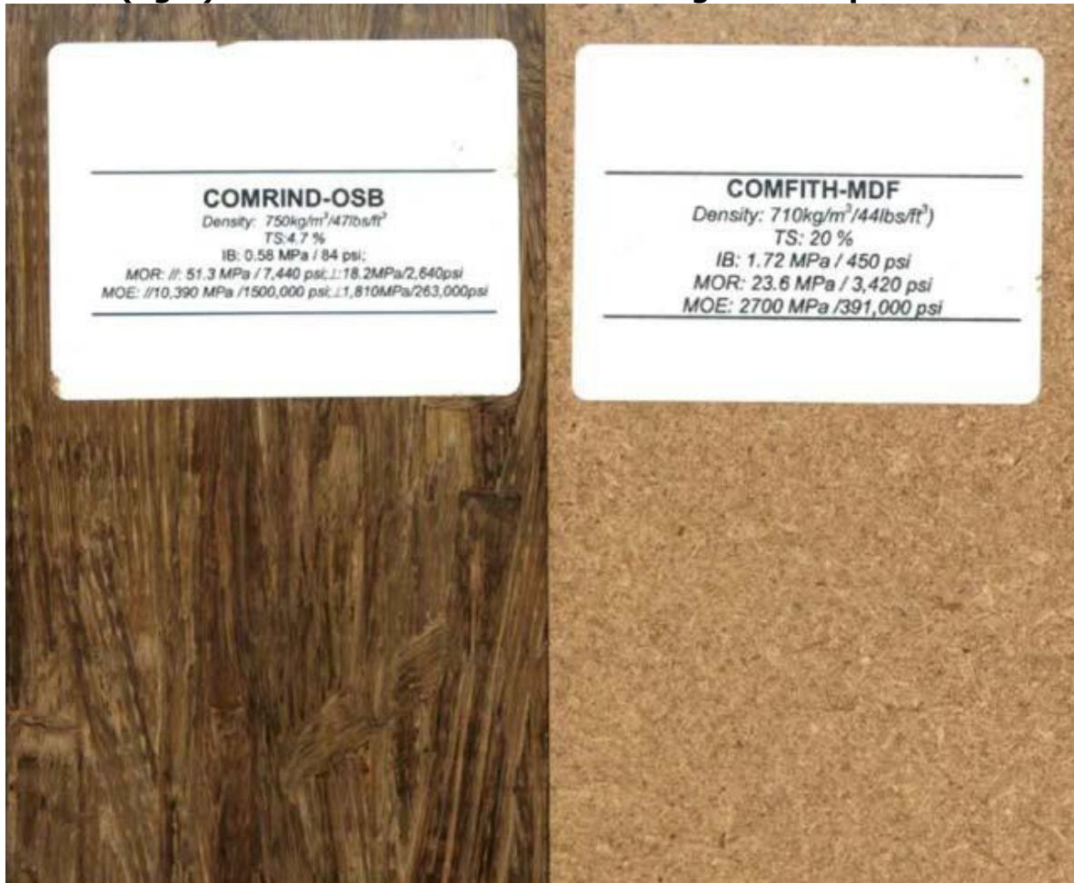
Figure 16: Oriented Strand Board From Comrind (left). Particle Board From Comfith (right). Board Products from Sweet Sorghum Components
