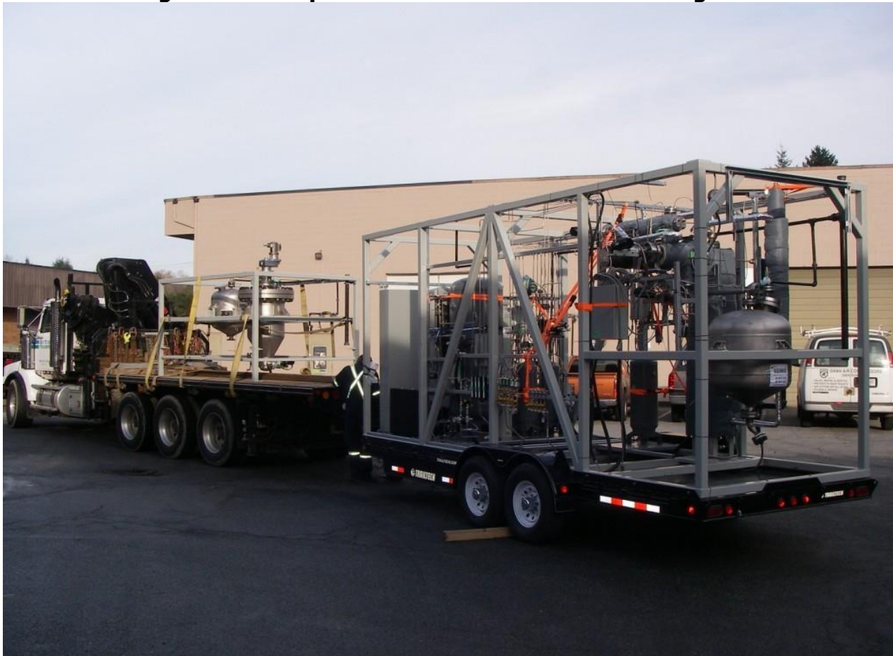
Figure 6: Transportation of DTU to Commissioning Site
