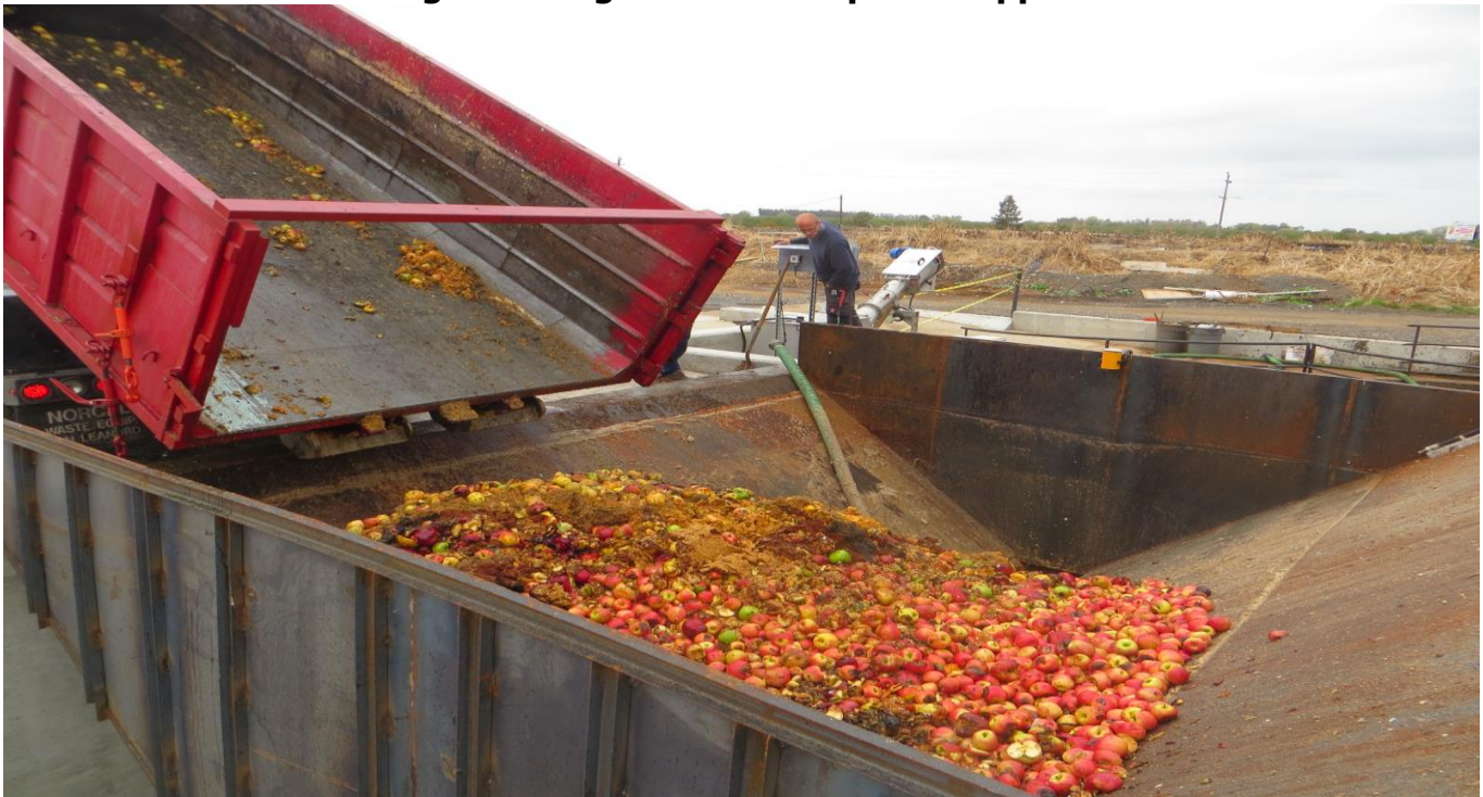
Figure 3: High Solids Reception Hopper
