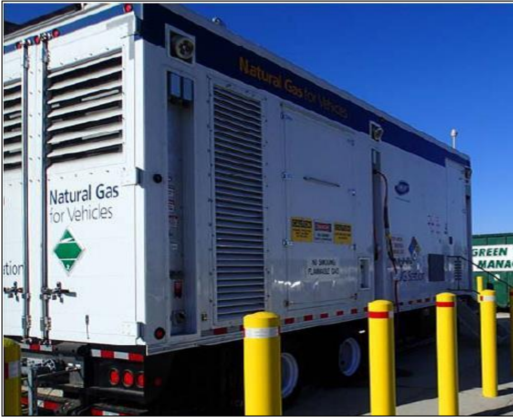
Figure 2: Portable Solution CNG Trailer
