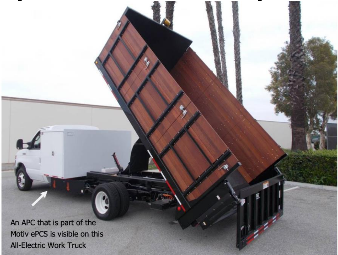
Figure 8: A Work Truck Built on the Ford E450 Chassis Using the Motiv ePCS
